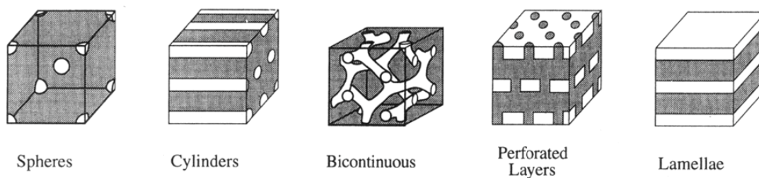
Figure 1.8. Schematic diagram of five different ordered microstructures observed for a series of polyisoprene-polystyrene diblock copolymer. Reprinted with permission from [42]. Copyright 1995 American Chemical Society.
