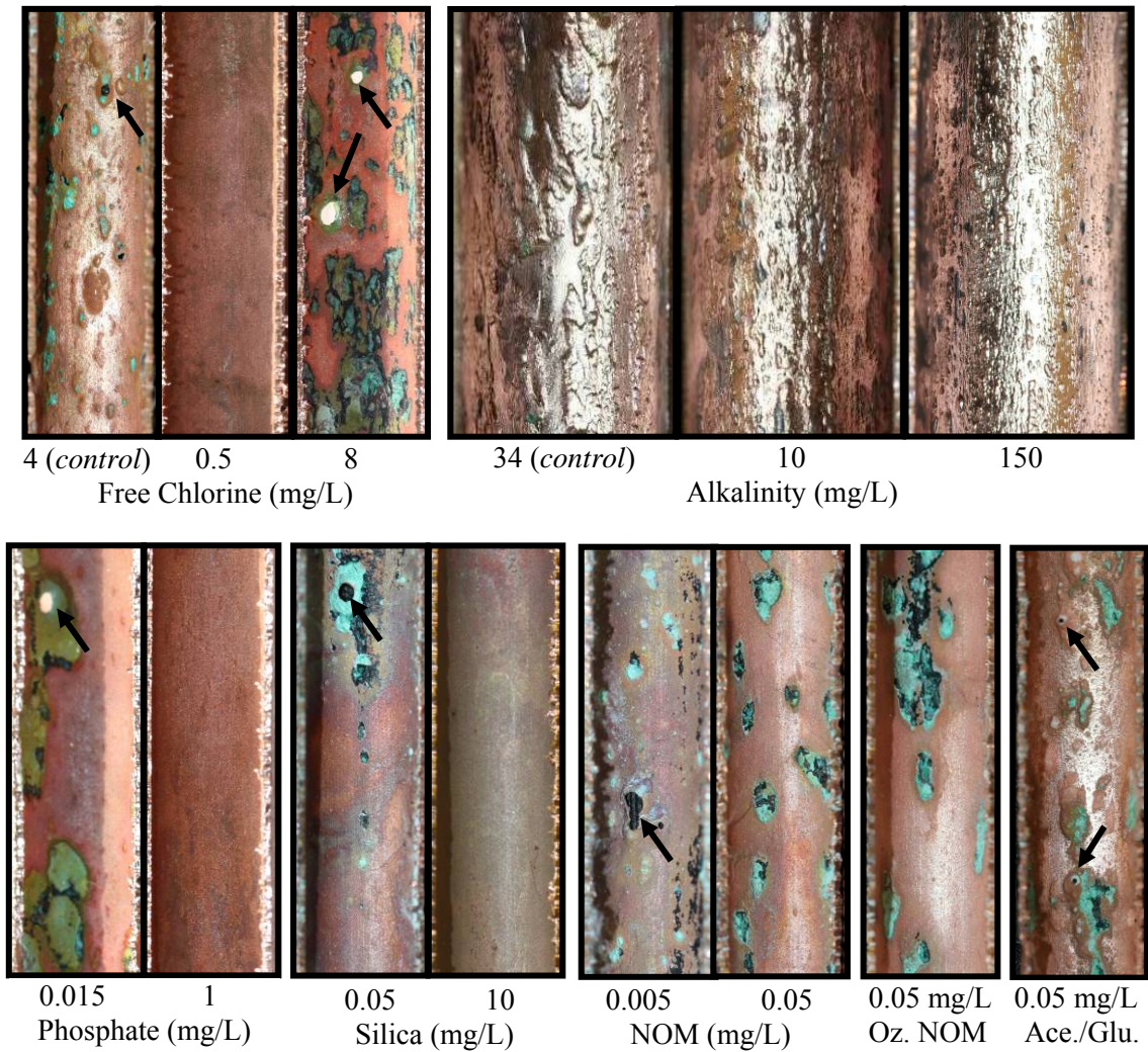
Figure 2.4: Representative photographs of copper from selected tests following scale removal. Photos are grouped by respective adjustments to control water quality, and arrows indicate some of the pinhole leaks that formed during testing. All photos show copper from small-scale tests, except for those in the variable alkalinity group.
