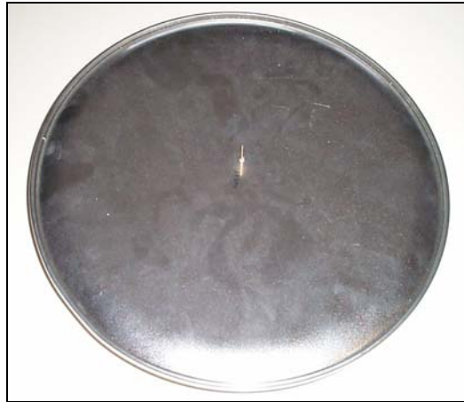
Figure 3.14. 5.0 GHz monopole antenna on a 6\lambda circular ground plane
