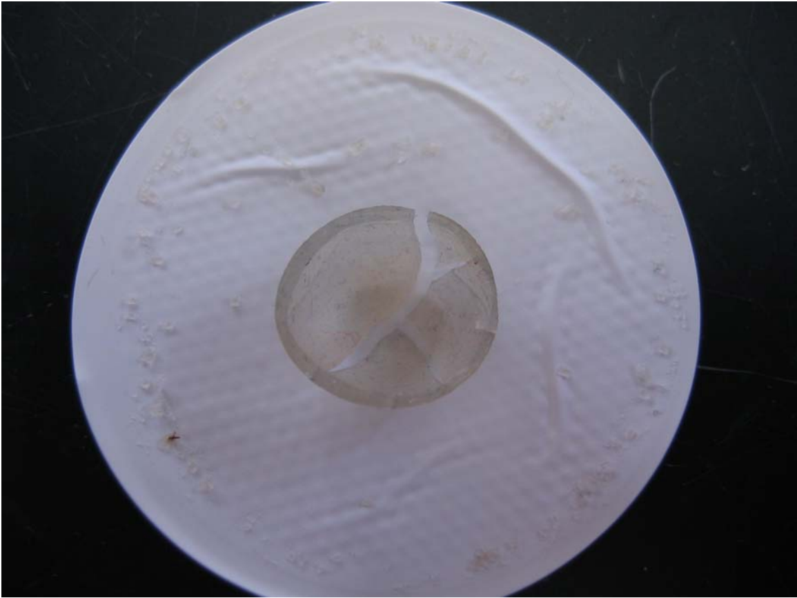
Figure 4-2. Air-dried filtered solid from pH 10.8 solution which originally contained 50 mg/L magnesium and 25 mg/L silicon.
