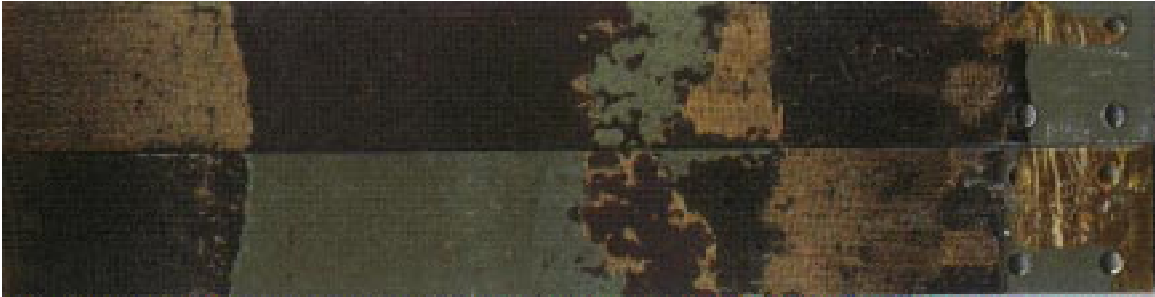
Figure 5.9. Photograph of the failure surface of an ENF test specimen showing interfacial failure.
