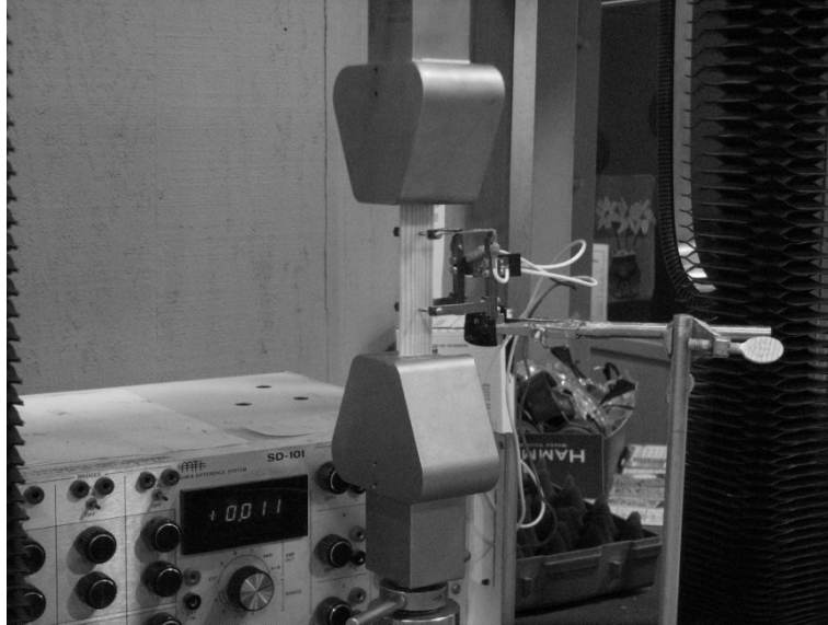
Figure 1. Tensile Testing of Wood Strands
