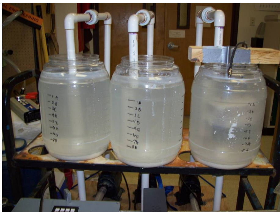
Figure 3.1. Sediment suspension system consisted of three plastic chambers, three submersible pond pumps, and three PVC piping networks.
