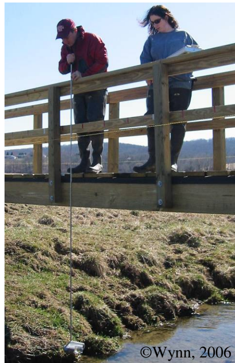
Figure 2.2. Barbra Utley and Alan Simpson during a training seminar in March 2006. Simpson was demonstrating proper usage of a depth-integrated D-48 isokinetic bottle sampler.
