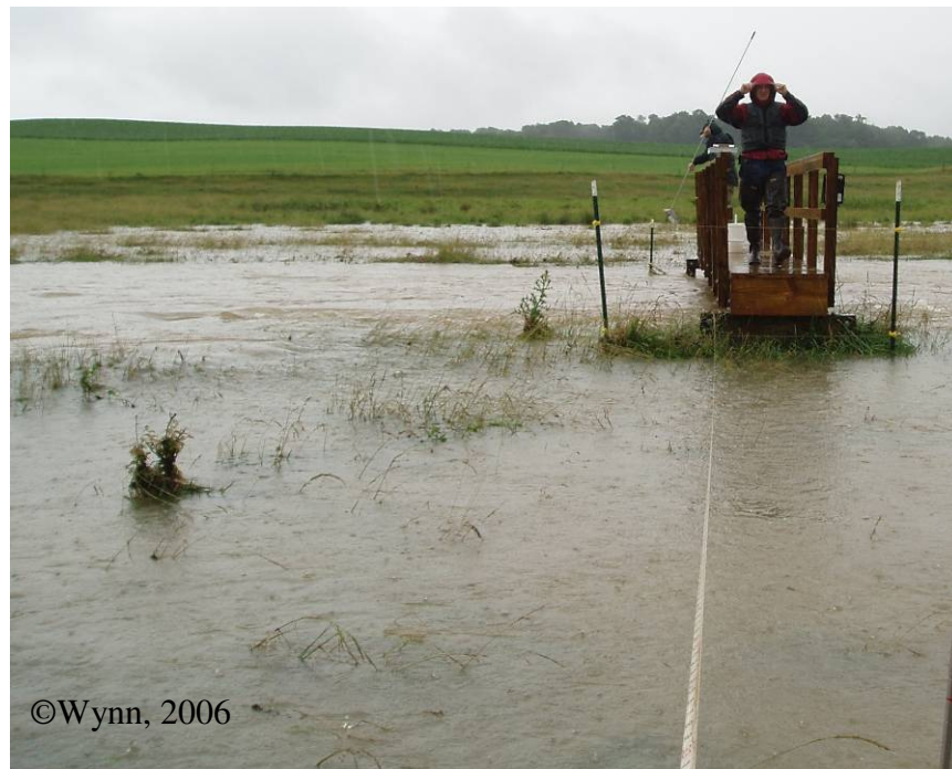
Figure 1.1. BSE graduate students sampling suspended sediment and measuring stream discharge during a storm event in June, 2006 on Stroubles Creek in Blacksburg, VA. The wooden bridge spans the bankfull stream channel.
