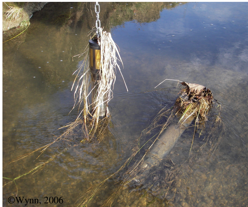
Figure 2.3. Eureka Manta sondes with turbidity probes in Stroubles Creek, on the Heth Farm, Blacksburg, VA. Two sensors are deployed to measure suspended sediment near the bed and near the surface of the water column.
