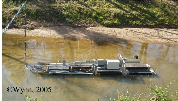
Figure 2.6. In-stream acoustic and depth-integrated pump sampling system developed by the U.S. Department of Agriculture, Agricultural Research Service in Gibson Creek near Oxford, MS, USA.
