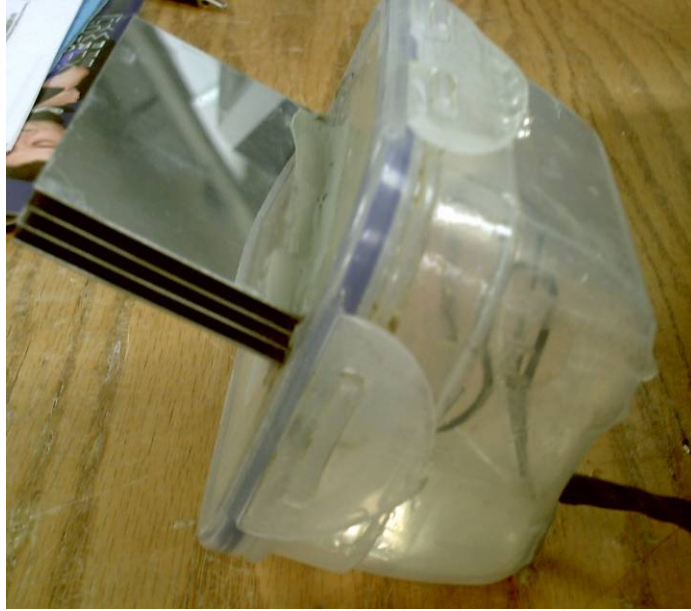
Figure 4.1. Permittivity electrode with plates made of 22 gauge, stainless steel with a plate spacing of 3 mm.
