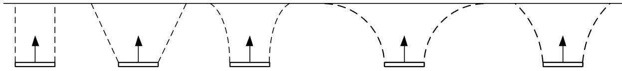
Figure 2.4 Idealized shapes of failure surface for shallow mode of failure. Left to right: cylinder, cone, trumpet, circular arc, log spiral
