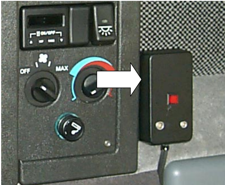
Figure 19. Nightcap interface unit located in the Volvo sleeper berth.
