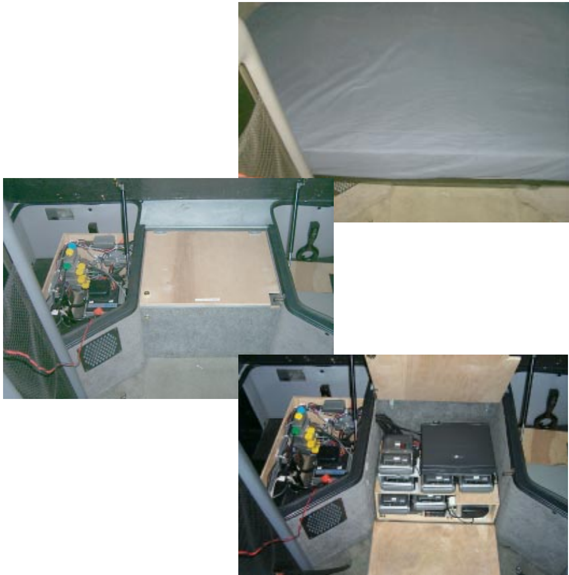
Figure 9. Instrumentation concealed in locked compartment (Middle Left) under the bunk in the Volvo (Bottom Right). Access is gained from inside the sleeper berth by lifting the mattress platform (Top Right).
