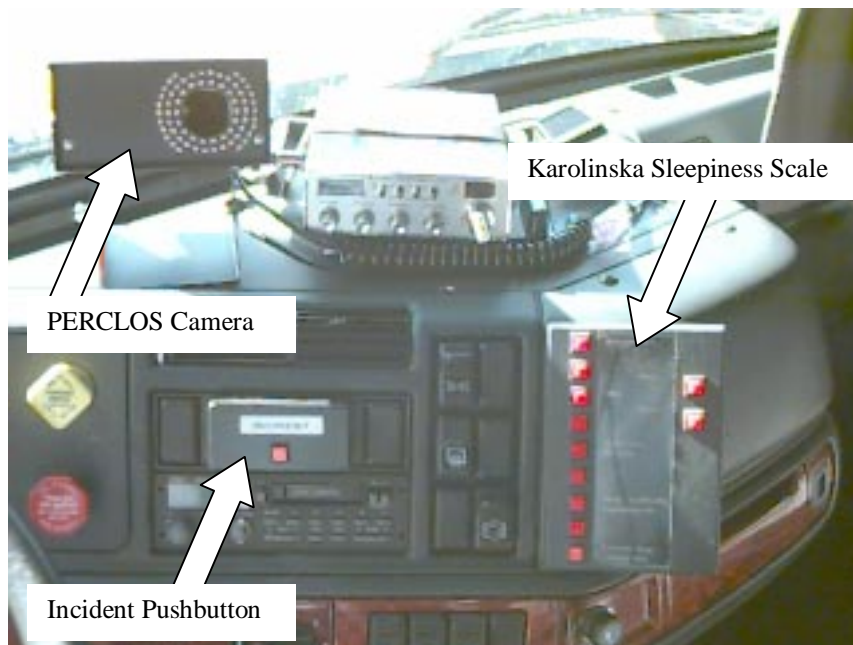
Figure 22. A view of the Volvo dashboard showing the showing the locations of the pushbutton used to trigger driver-initiated critical events, the Karolinska sleepiness scale, and the PERCLOS camera.
