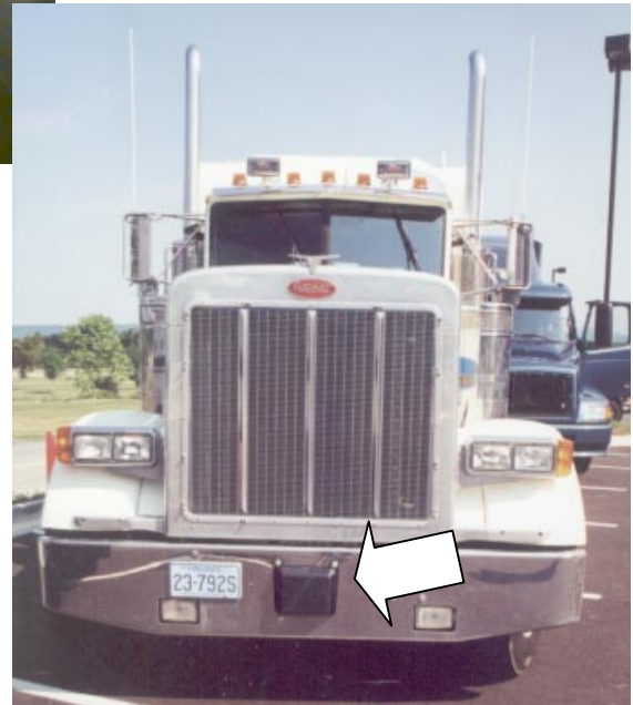
Figure 14. Eaton Vorad side clearance sensor (Top Left – passenger side shown) and headway sensor (Lower Left) mounted on the Peterbilt.
