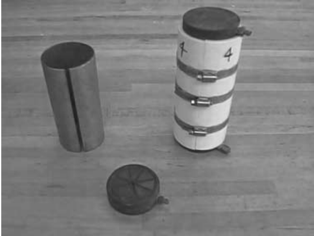
Figure 6-3 From left to right, stainless steel mold, platen, and PVC mold for forming stabilized sand samples
