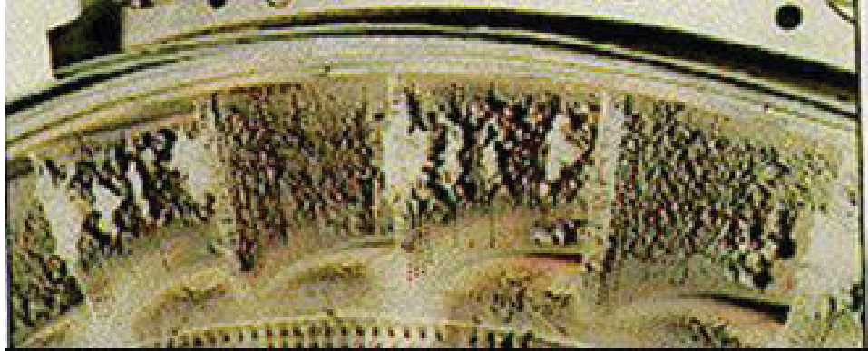
Figure 1.2. Image of turbine nozzle guide vanes after ingestion of volcanic ash.
