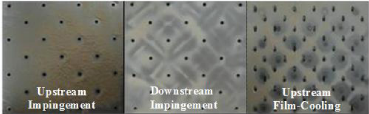
Figure 1.12. Post-test images of sand deposition patterns at ambient temperature for L1 at PR=1.03.
