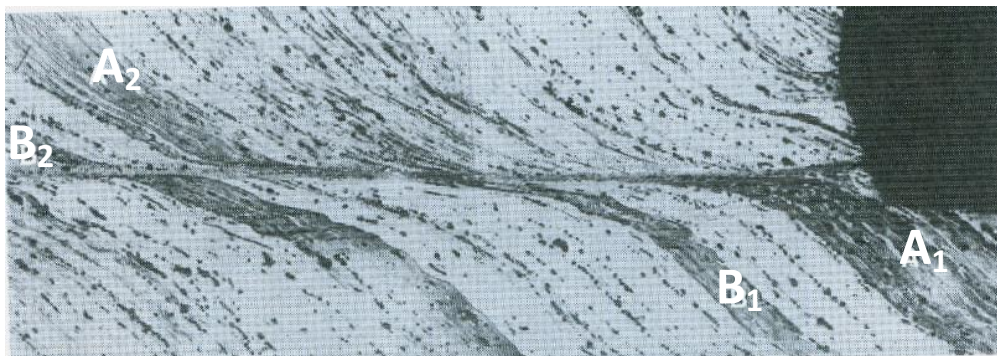
Figure 2.1: ASB in a 2014-T6 Al alloy formed at the corner of a crater. Source: Wingrove [1].
