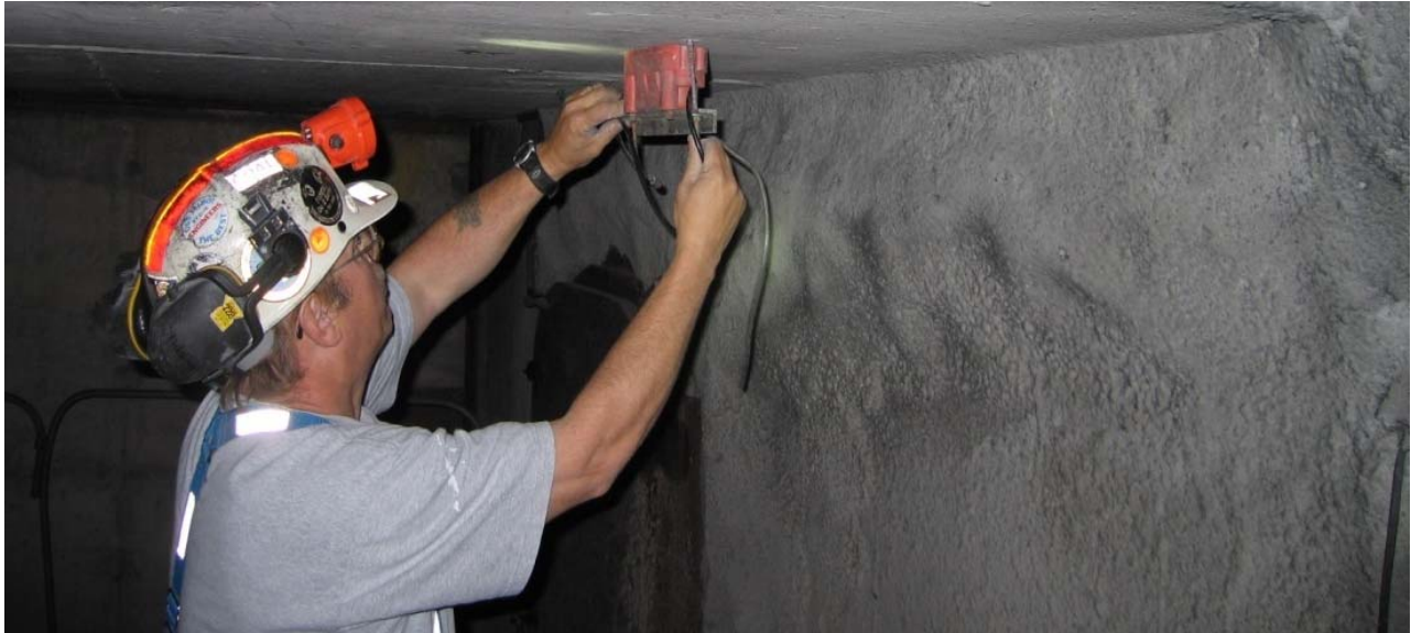
Figure 3.9 – Photograph of the geophone used in the study. In the photograph, the geophone is being installed at the test site.
