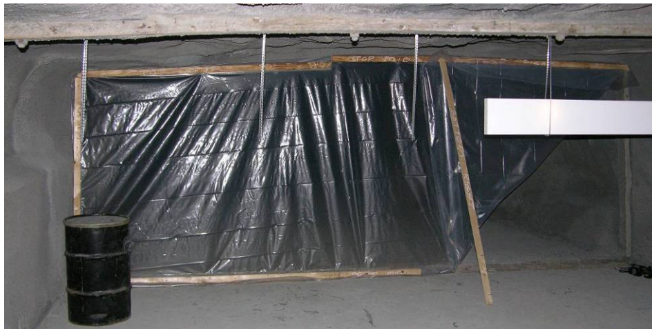
Figure 3.20 – Plastic diaphragm used to contain the methane within the ignition chamber.
