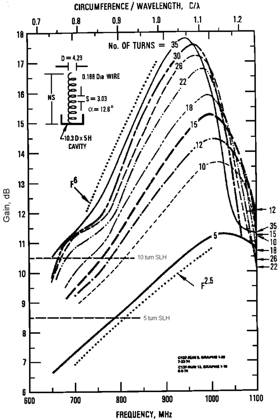
**Figure 8.1** Antenna gain versus frequency for 5- to 35-turn helical antennas, 4.23-in diameter. The curves are from [King and Wong, 1980]. The horizontal dashed lines indicated average SLH gains for 5- and 10-turn models based on NEC modeling presented in the preceding sections.
