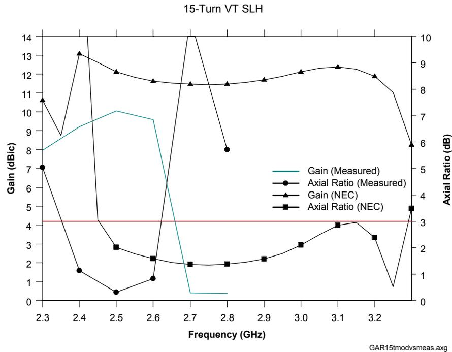
**Figure 8.3** Gain and axial ratio measured for 10-turn S-band prototype P15-1 and simulated using NEC model M15-1.
