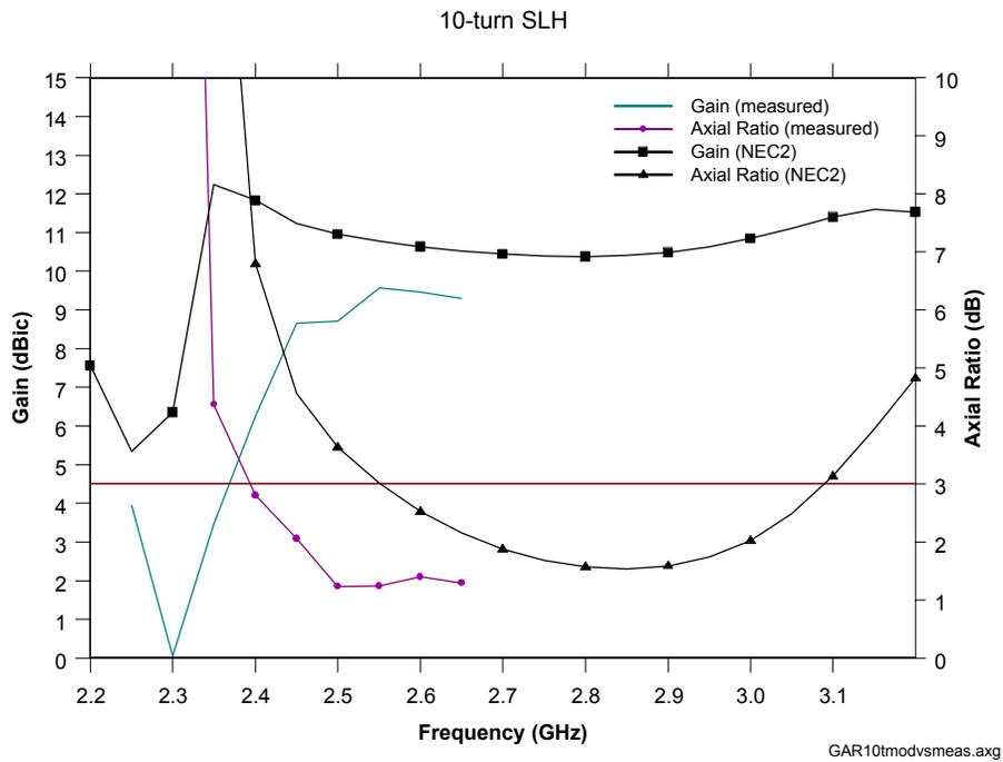
**Figure 8.2** Gain and axial ratio measured for 10-turn S-band prototype P10-1 and simulated using NEC for model M10-3.
