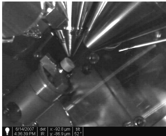
Figure 3.4. The FIB – SEM position of sample relative to the two beams.
