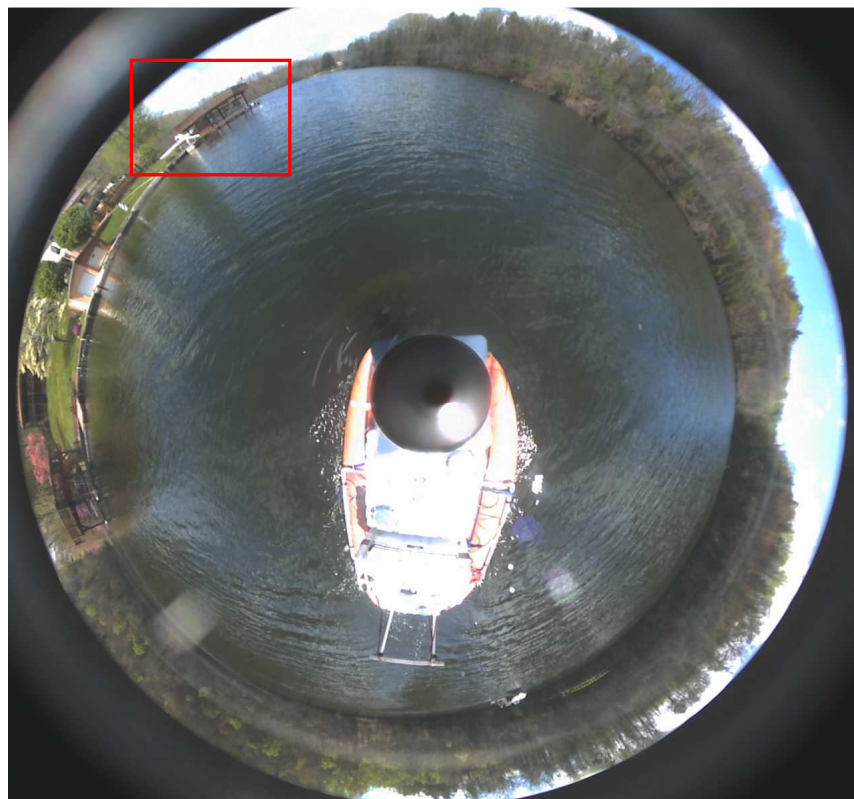
Figure 6.14: The dock marked by red rectangular was detected as obstacles.
