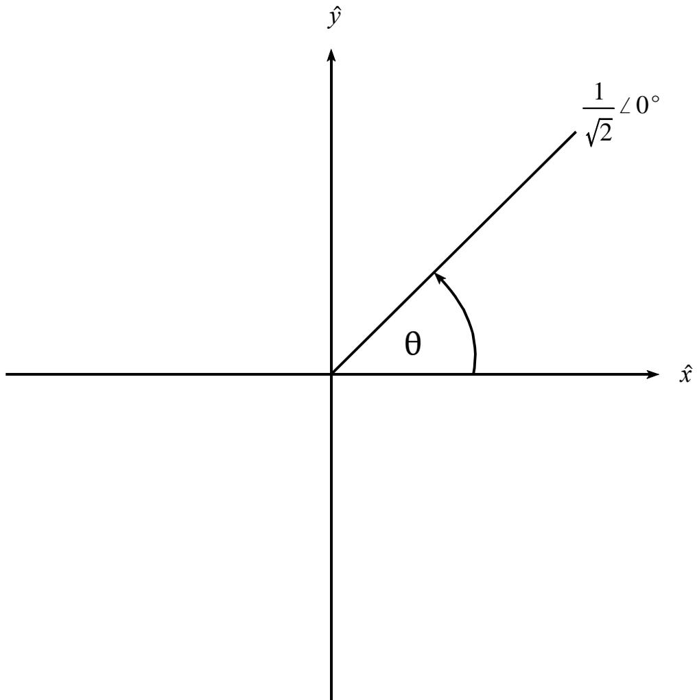
**Figure B.1 Polarization-Phase Representation of a Rotating LP Antenna**
