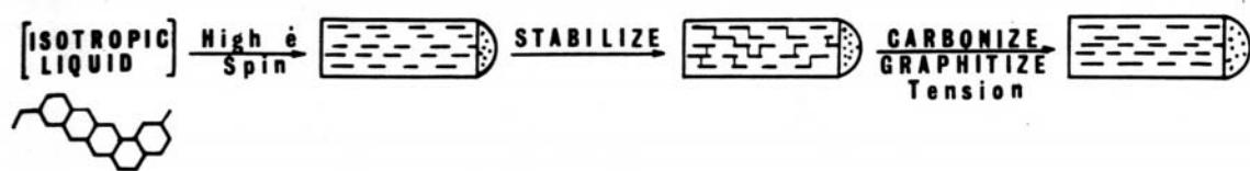
**Figure 2.3:** Schematic of isotropic pitch processing steps<sup>10</sup>.
