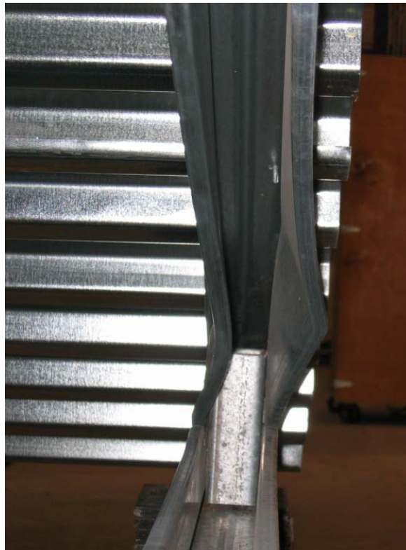
Figure 5.9 T1C Test 1 Distortional Buckling Failure
