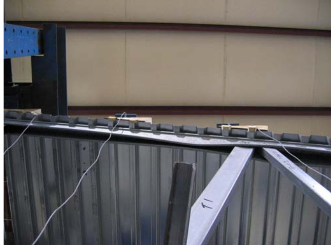
Figure 5.14 Distortional Buckling of 5-in Top Chord Member
