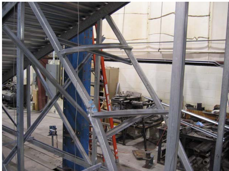
Figure 5.12 T1 Test Out-Of-Plane Buckling due to Initial Imperfection
