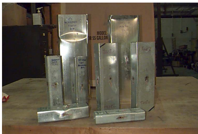
Figure 3.4 Failure of all specimens
