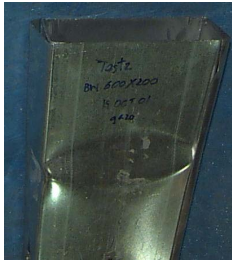
Figure 3.3 Typical Inelastic Local Buckling Mode of Failure
