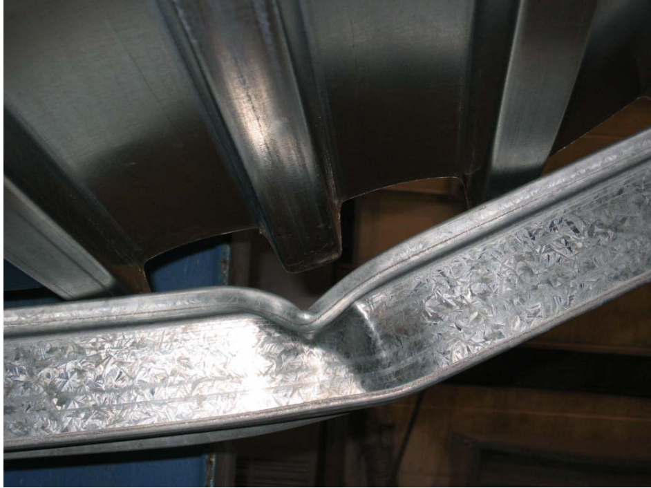
Figure 5.7 T1A Test 2 (Second Run) Combined Compression and Bending Failure
