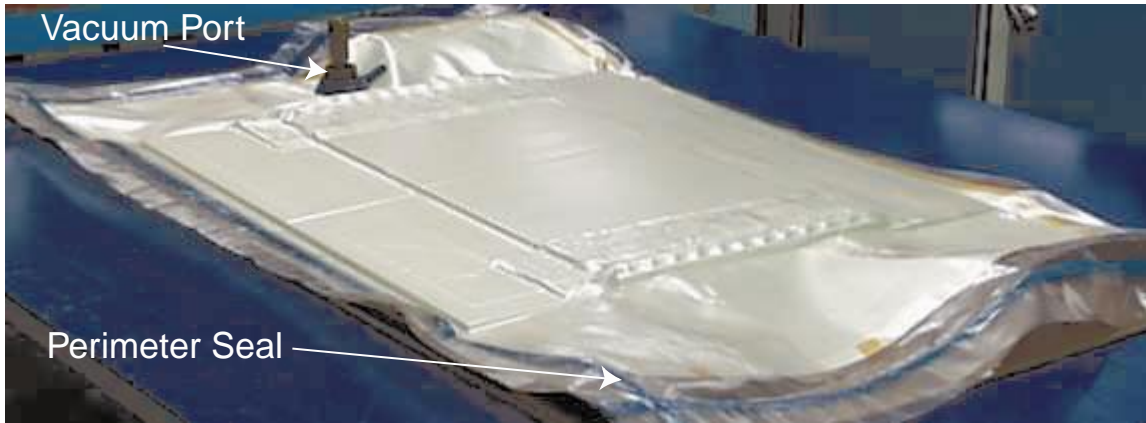
Figure 3.8 Laminate after vacuum-bagging and applying vacuum.
