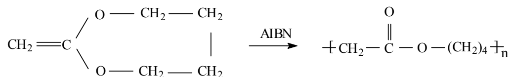
Figure 11.3 Ring opening polymerization of 2-methylene-1,3-dioxepane (MDO) to produce poly ( \epsilon -caprolactone).
