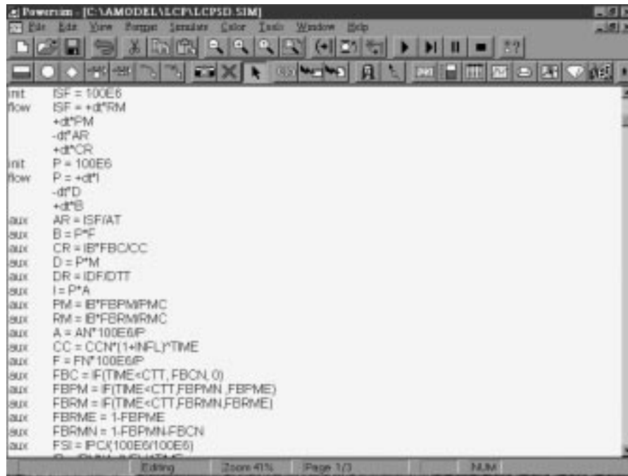
Figure 8.9 Systems equation of LCPSD model using Powersim
