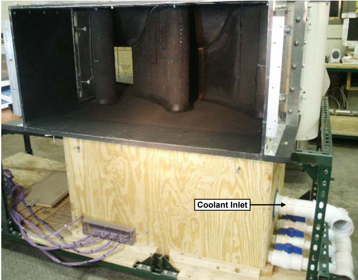
Figure D.6 Illustration of the endwall coolant plenum showing the single coolant supply line (the other inlet pipes that are shown were blocked and not used).
