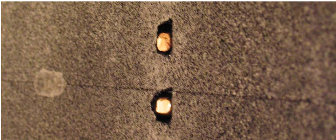
Figure D.3 Example of two non-circular holes at the metering area. The upper hole has an ovular shape, while the lower left-hand quadrant of the lower hole was approximated as a square.
