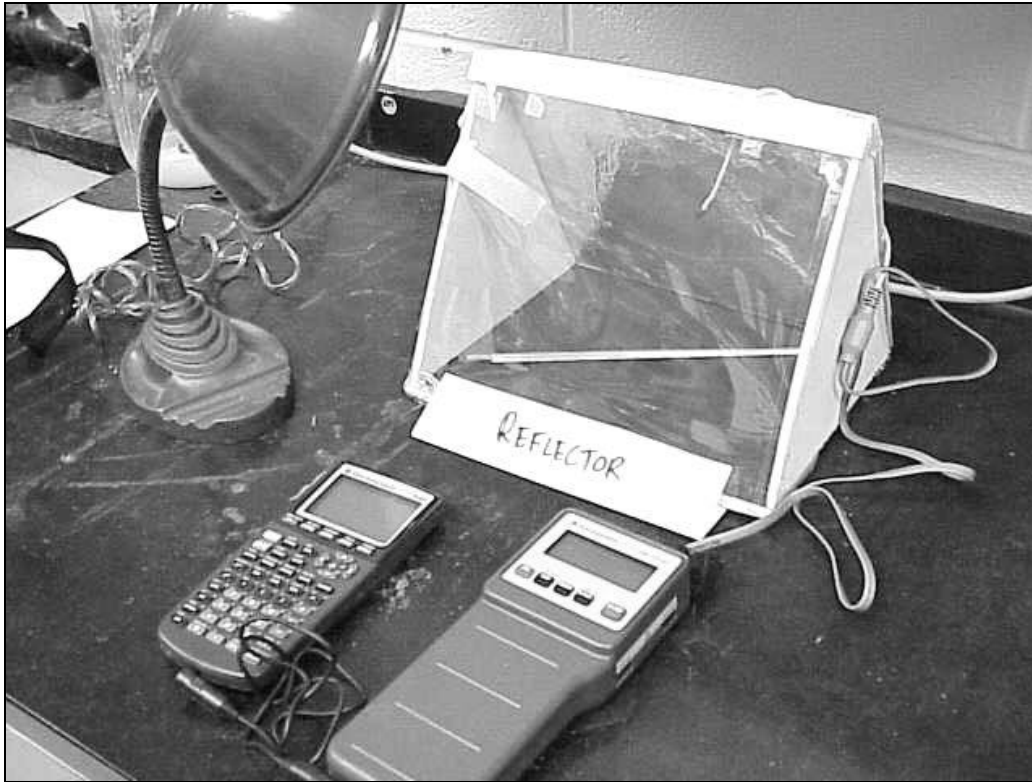
Figure B. Lab apparatus including solar house model, graphing calculator (left), CBL, temperature probe, and gooseneck lamp. The model has a black, construction paper floor and a mirror on the back wall.
