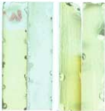
Figure 89. Digital photographs of the CAVE networks cured with 30 % methyl methacrylate and BPO (80°C for 1 hr, then 100°C for 1 hr). For each of the two pairs of samples, the aged is on the left and the control is on the right. The left pair is a top view (exposed side) and the right pair is a side view.
