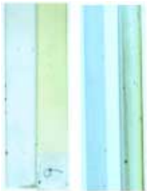
Figure 91. Digital photographs of the bisphenol-A vinyl ester networks cured with 30 % styrene and BPO. For each of the two pair of samples the aged is on the right and the control is on the left. The left pair is a top view (exposed side) and the right pair is a side view.
