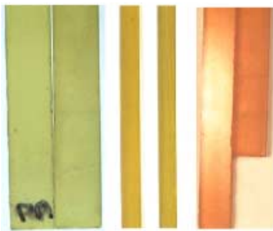
Figure 88. Digital photographs of the CAVE networks cured with 40 % methyl methacrylate via methyl ethyl ketone peroxide, cobalt naphthenate, and dimethylaniline. For each of the three pair of samples the aged is on the left and the control is on the right. The left and right pairs are top views (exposed side) and the center is a side view.
