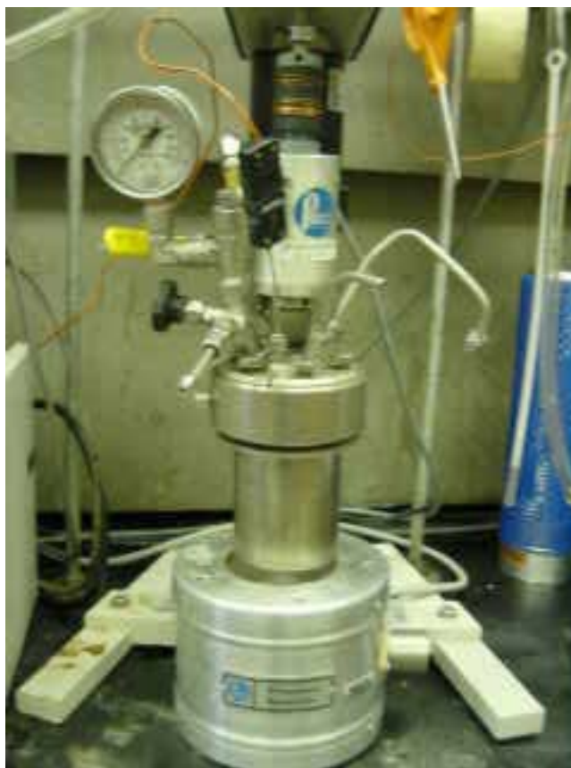
Figure 4.2-3: A closer look at the configuration of the Parr Reactor
