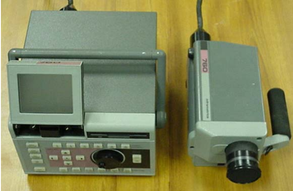
Figure 4.25 Photograph of the Inframetrics Model 760 infrared camera and controller used for thermal mapping of the vane passage endwall.
