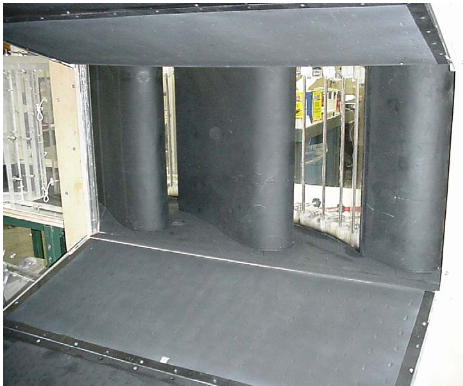
Figure 4.13 Baseline unfilleted, slotless combustor simulator configuration.
