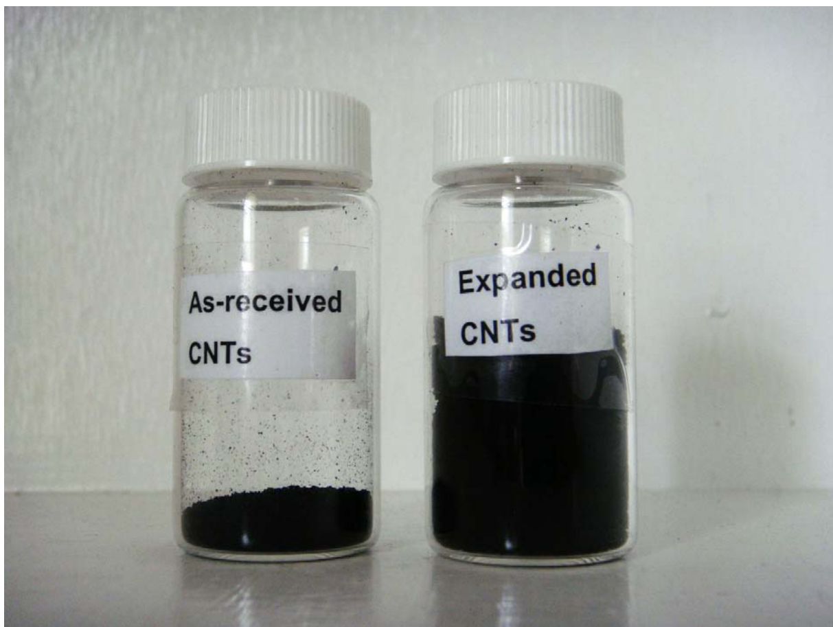
Figure 3.1: Photo picture of carbon nanotubes with same weight (0.10g) before (left) and after (right) expansion using supercritical CO 2
