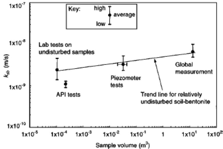
Figure 2-2 The influence of sample size on the resulting value of hydraulic conductivity (after Britton et al. 2004, with permission from ASCE)
