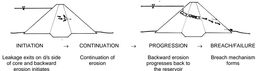
Figure 2-7 A four-phased model for the development of piping failure initiated by backward erosion (after Fell et al 2004, with permission from the University of New South Wales).
