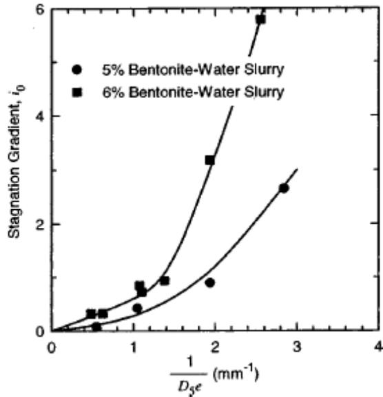
Figure 2-4 Chart for estimating stagnation gradient,  $i_0$ , of slurry (after Filz et al. 2004, with permission from ASCE)
