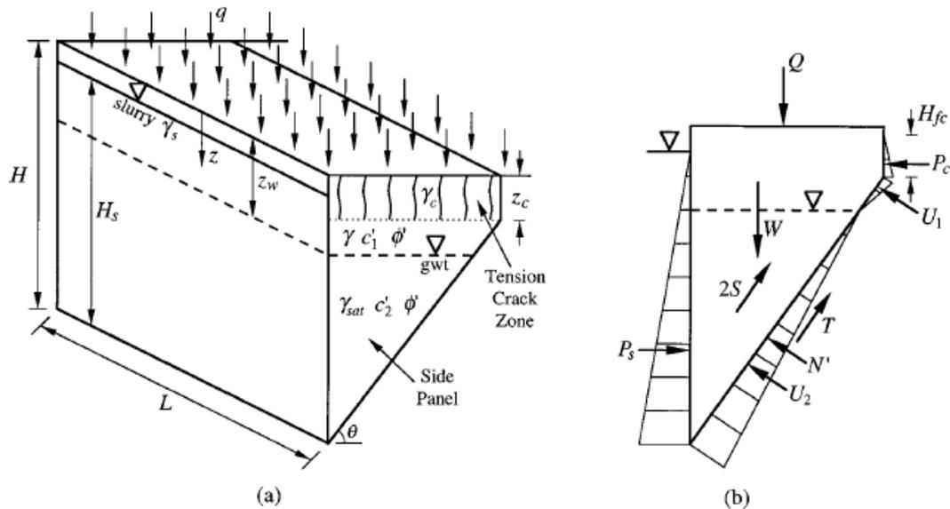
Figure 2-5 Geometry (a) and forces (b) on a failure wedge into a slurry-supported trench with a tension crack above the groundwater table (after Fox 2004, with permission from ASCE)
