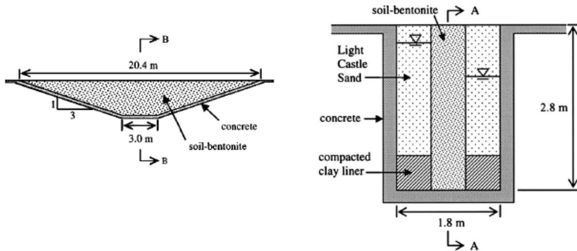
Figure 2-1 Longitudinal (left) and transverse (right) profiles of barrier pit and soil-bentonite barrier (after Britton et al. 2004, with permission from ASCE)
