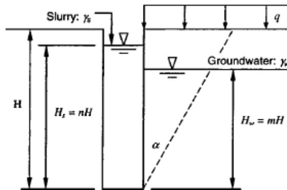
Figure 2-3 Definitions of variables for global stability of a trench where a filter cake has formed (after Filz et al. 2004, with permission from ASCE)
