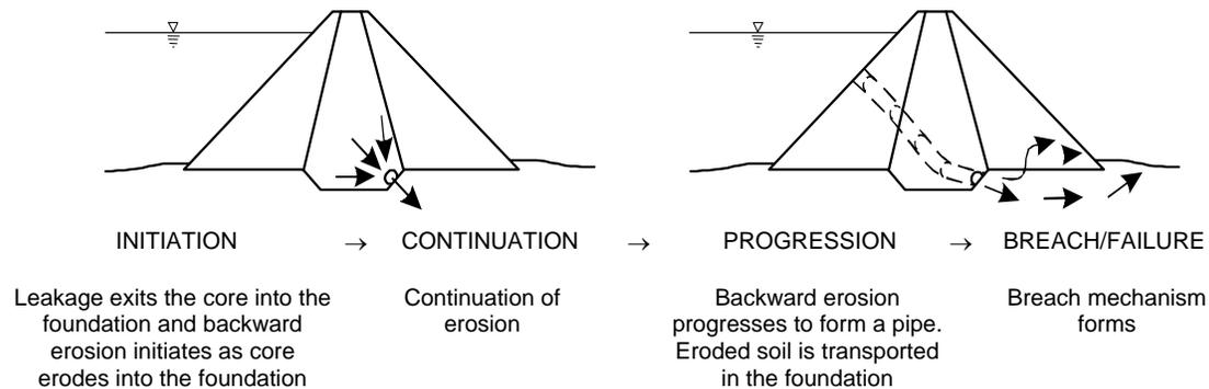
(B) PIPING FROM THE EMBANKMENT TO FOUNDATION INITIATED BY BACKWARD EROSION
