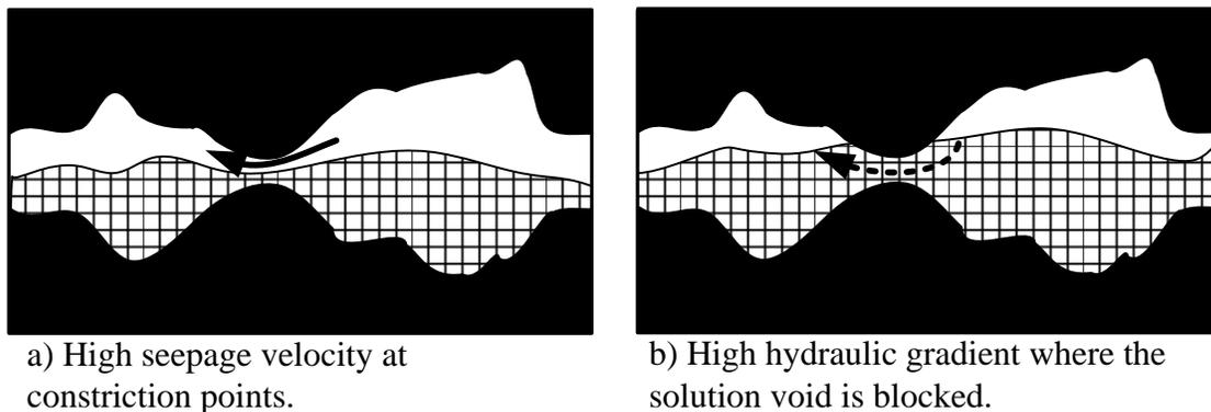
Figure 5-5 Schematic illustration of increased erosion potential in solution voids
