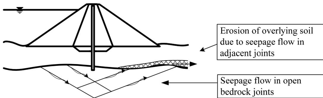
Figure 5-4 Erosion of adjacent soil due to seepage flow in bedrock joints
