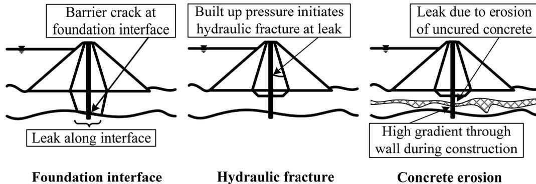
Figure 5-2 Conditions where coincidence of barrier defects and concentrated seepage pathways are likely.
