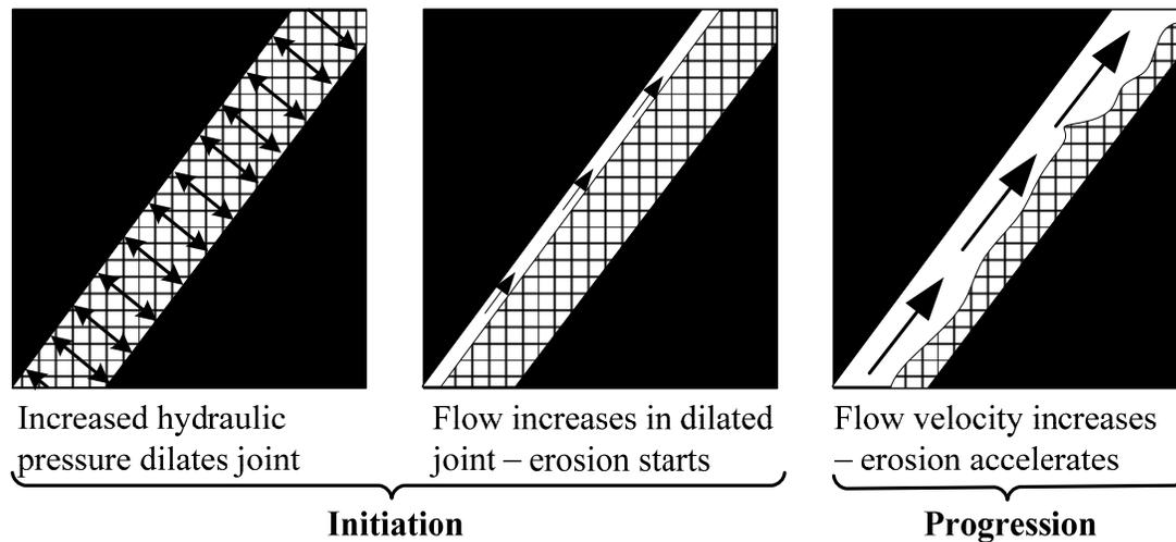
Figure 5-3 Erosion of soil through bedrock joints
