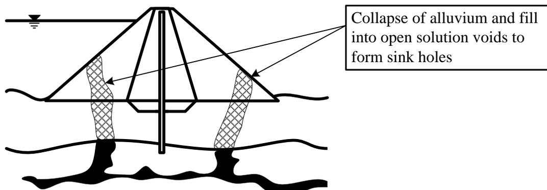
Figure 5-6 Collapse of overlying soils into open solution voids
