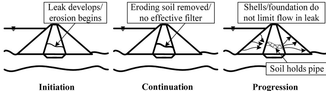
Figure 5-1 Phases of development for internal erosion and piping (modified from Fell et al. 2004 and Foster and Fell 1999, with permission from University of New South Wales)
