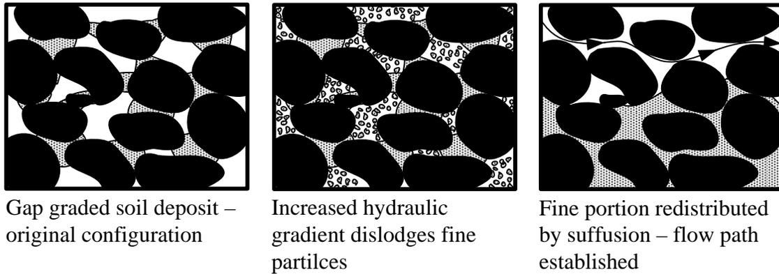
Figure 5-7 Development of concentrated flow pathway by suffusion
