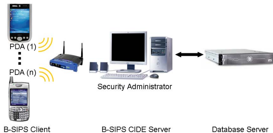
Figure 4-5 B-SIPS System Design
