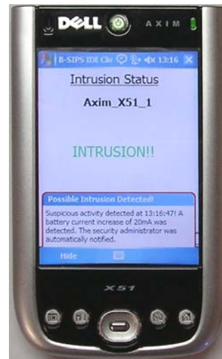
Figure 6-32 B-SIPS Report of Threshold Breach on Dell Axim X51
