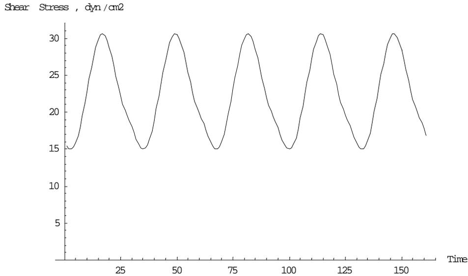
Figure 2. Calculated shear stress from pressure drop measurements. Pressure drop data obtained during cell culture in the Cellmax® capillary system were used to calculate the time-dependent wall shear stress. Shear stress was obtained from the gradient of the velocity profile at the wall determined from the Womersley solution of the Navier-Stokes equation.
