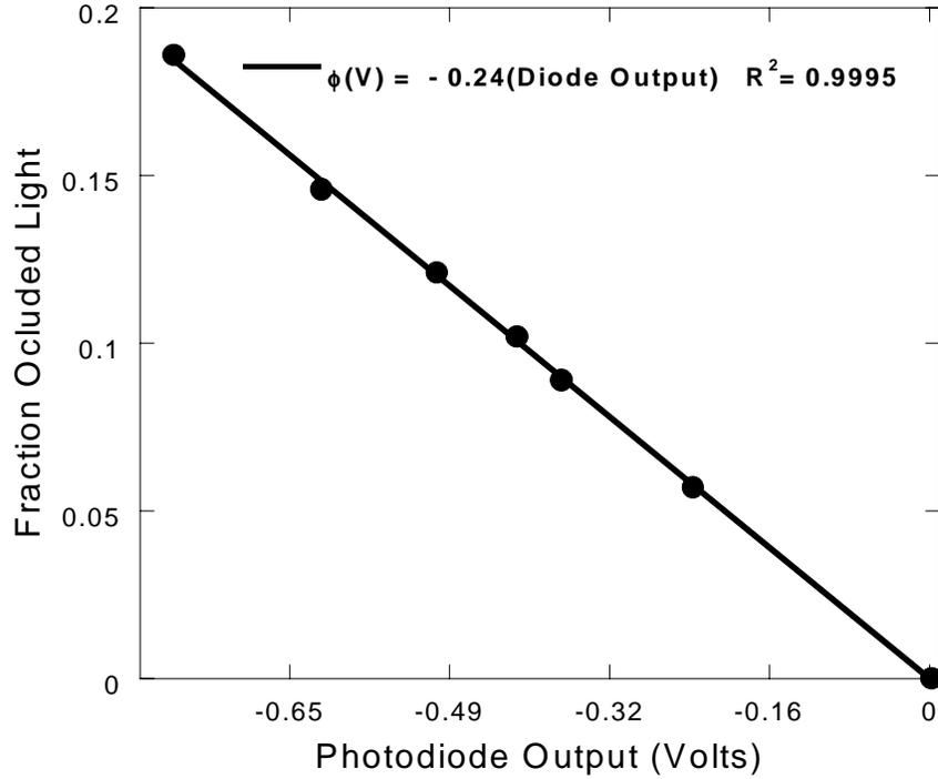
Figure 5. Calibration curve for the laser occlusion apparatus. The test polypropylene capillary (630  $\mu\text{m}$  OD, 330 $\mu\text{m}$  ID) was used to calibrate the photodiode output to the fraction of laser light occluded, which can then be related to the vessel radius using Eq. 2. The change in fraction of light occluded was achieved by positioning the capillary at specified intervals between the lens and the photodiode, and the fraction of light occluded calculated using Eq. 1.
