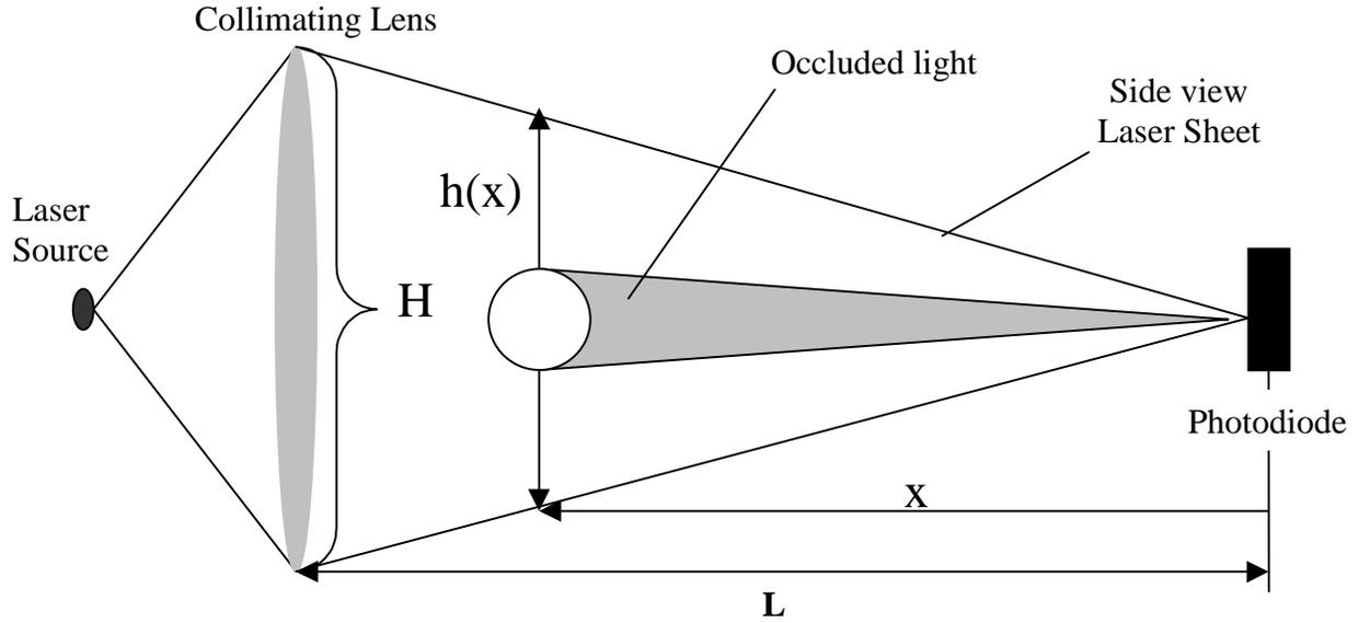
Figure 4. A schematic of the cross sectional view of the laser light geometry describing the fraction of laser light occluded.  $H$  represents the lens height,  $x$  the varying distance from the diode to the sample position,  $h$  the effective laser beam height at position  $x$ , and  $L$  the fixed focal length.
