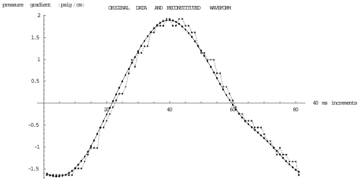
Figure 1. Fourier series representation of pressure drop data. Using a differential pressure transducer the pulsatile pressure drop across the cell culture capillaries was recorded (\*). One cycle of the data was then fitted to a harmonic series with 10 terms using DFT (◆). Note that the data was scaled by subtracting the contribution from the time averaged pressure drop component.
