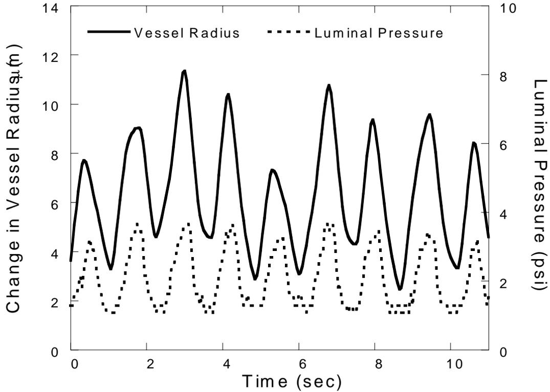
Figure 6. Measurement of a Pharmed® vessel distention under transluminal pressure gradient. A Pharmed® vessel was subjected to a manual transluminal pressure gradient and the vessel change in radius was measured using a laser occlusion non-contact optical method. This data set is representative of dynamic testing of the Pharmed® vessel (2.6 mm OD, 1.6 mm ID) under no luminal flow conditions and was repeated at least three times with three different vessels.
