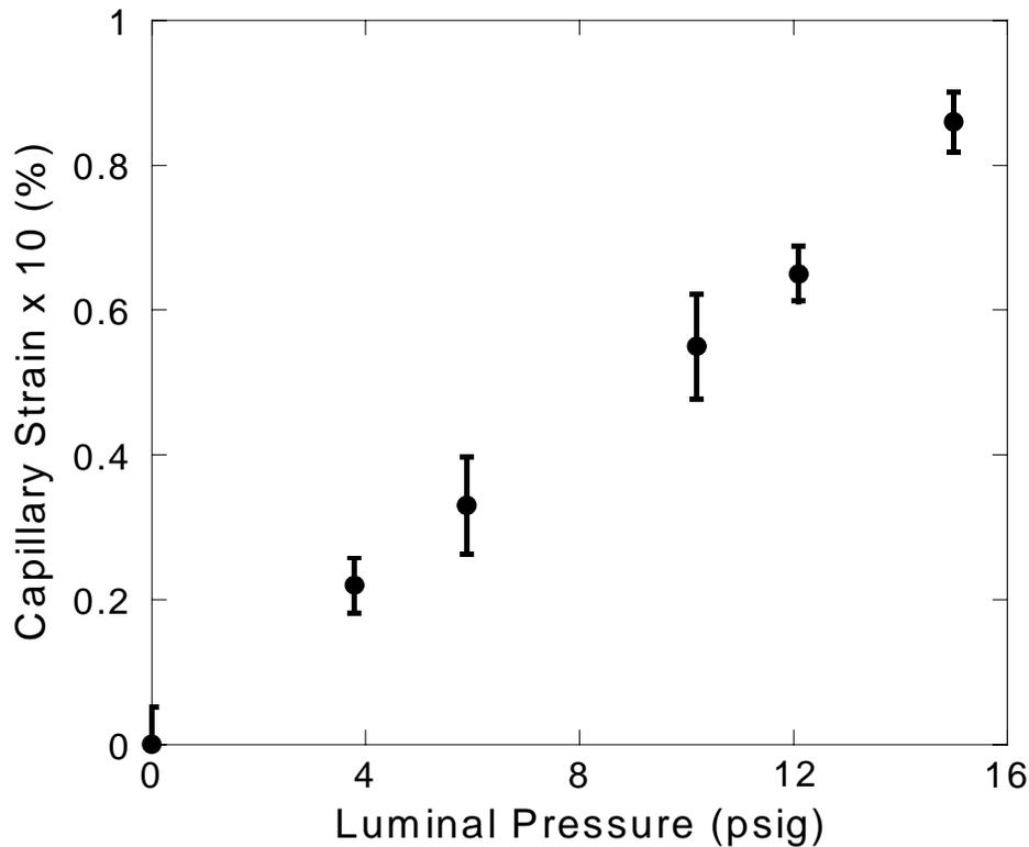
Figure 7. Strain vs luminal pressure plot for a polypropylene capillary. Polypropylene capillaries were tested under sustained luminal pressure driven flow (with a syringe pump). Pressure and capillary radius were measured using a pressure gage and the laser occlusion apparatus. Data points represent the mean  $\pm$  standard deviation for 8 separate capillaries. The error in pressure measurement is less than 0.01 psi (OMEGA, Inc., Stamford, CT).
