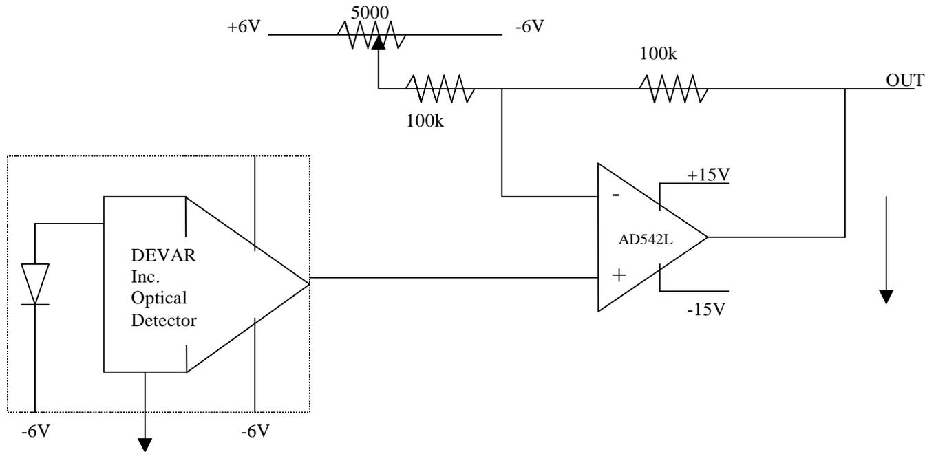
Figure 3. Optical sensor and amplifier circuit design. The photodiode uses  $\pm 6V$  excitation from a regulated power source and the output is an input to an op-amp and variable resistive circuit that allows baseline setting and scaling of the voltage output to the I/O board.
