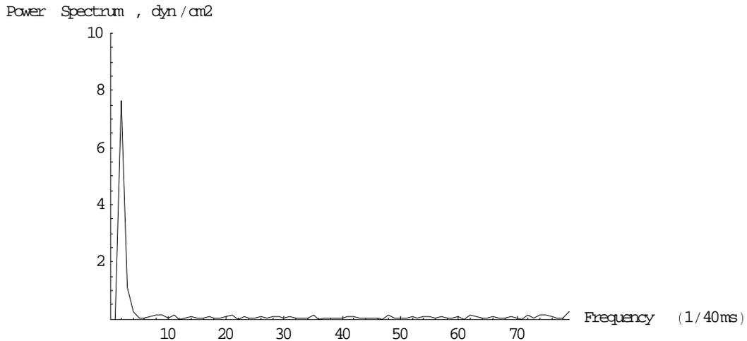
Figure 3. Power spectrum of the pressure waveform data. Pressure drop data were obtained during the high shear stress treatment in our cell culture system and analyzed using FFT. The sampling frequency was 25 Hz.
