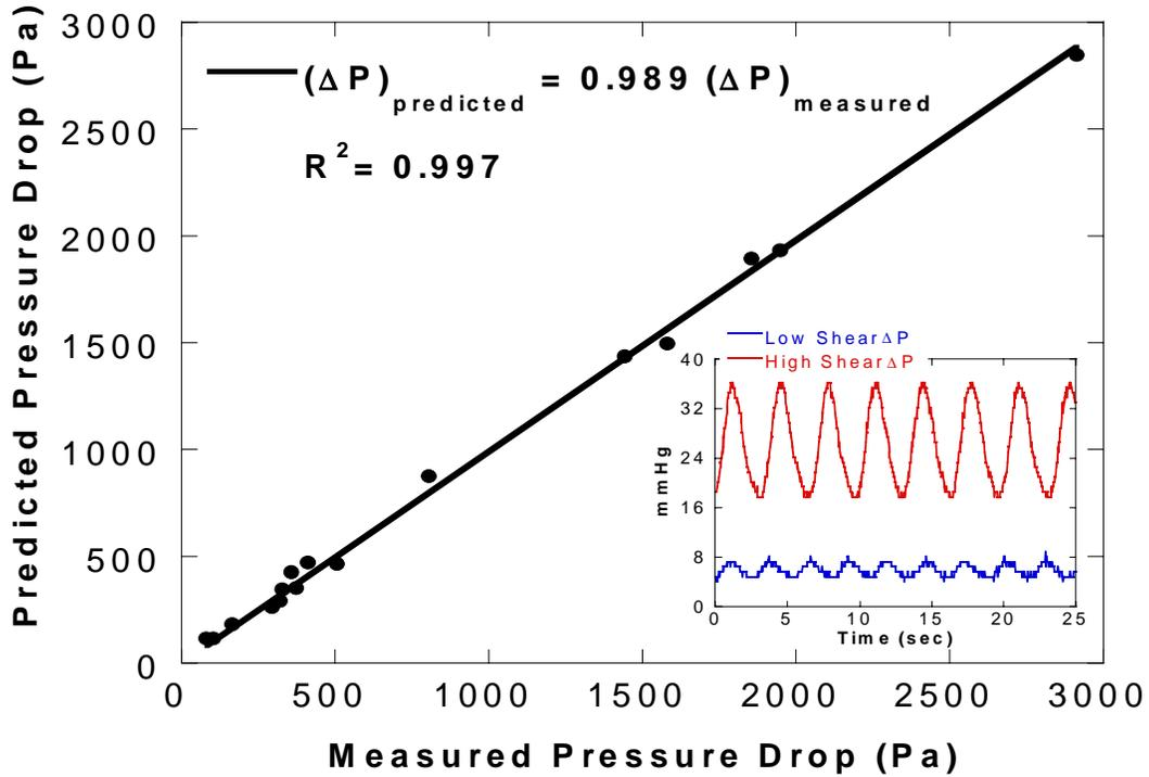
Figure 4. Pressure drop was calculated from the laminar flow equations and compared to average pressure drop measured for low and high shear experiments in our cell culture model. The pressure drops are equal indicating that the flow is laminar. Inset shows the measured pressure drops as a function of time for low and high shear experiments.
