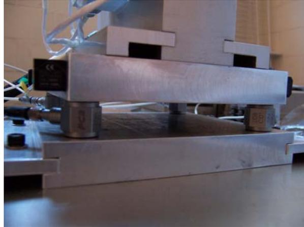
**Figure 3.15: Close-up photograph of force transducers and sandwich plates**
