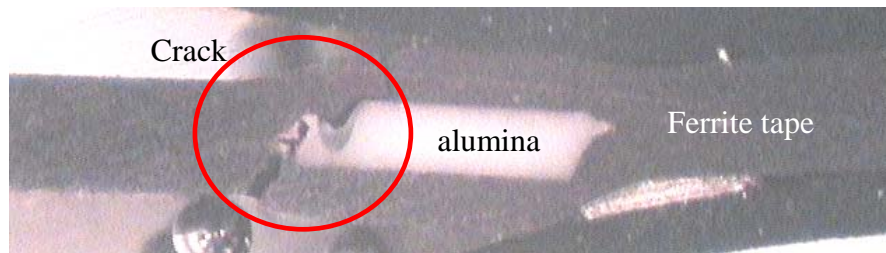
Figure 2-17 Cross-sectional view of a thin alumina strip sandwiched in LTCC ferrite tape after sintering.
