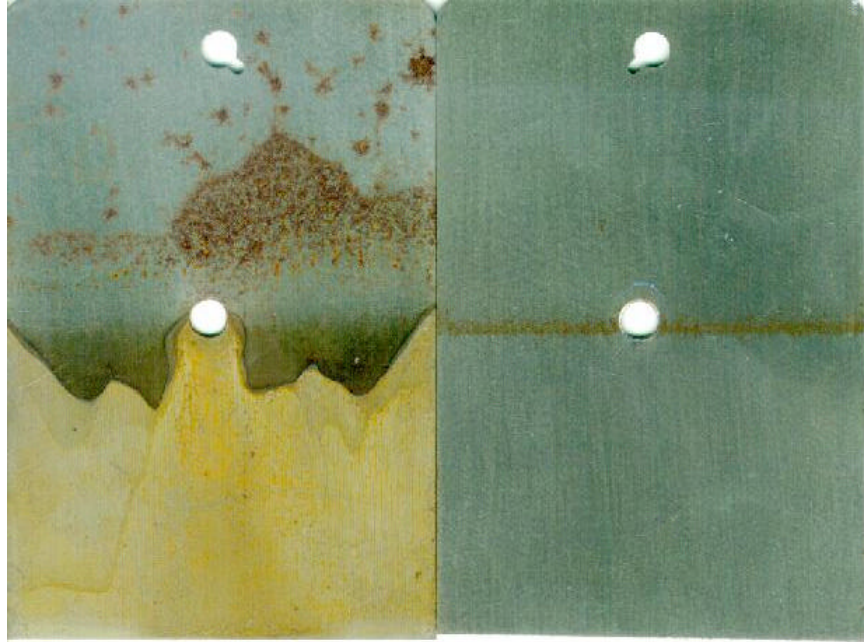
Figure 22. Comparison of the corrosion resistance of uncoated (left) and f-DETA(100) coated (right) steel. Samples were half immersed in salt water.
