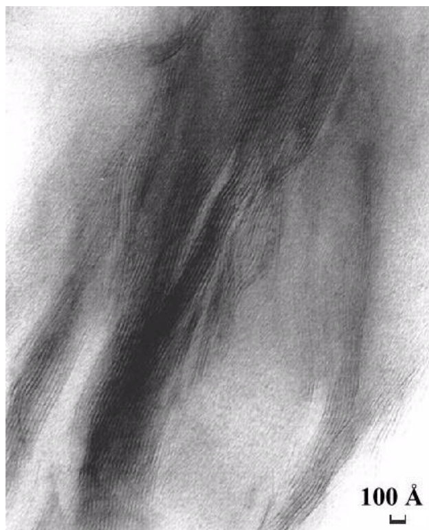
Figure 6. TEM image of an intercalated, cured epoxy system based on Epon828-D400 with PS3 organoclay.
