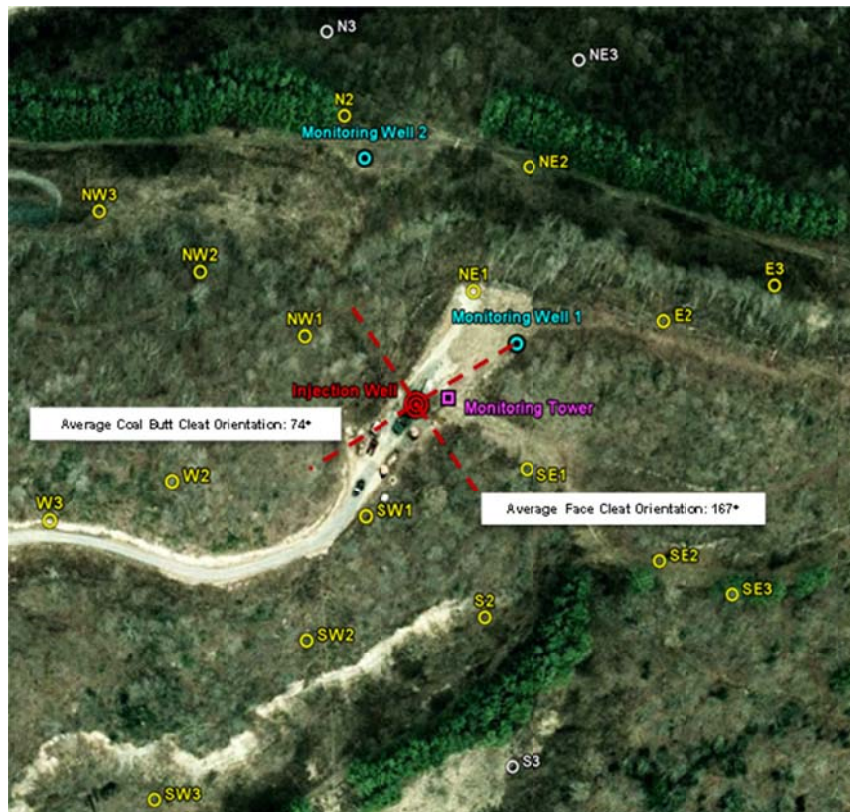
Figure 17: Field validation test site layout, Russell County, VA. (Aerial view) (Source: Google Inc. (2011). Google Earth (Version 6.1.0.5001))
