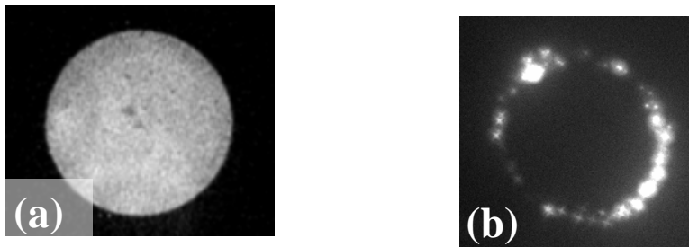
Figure 23. The electroluminescence image on the CCD camera corresponding to a 1.12 cm diameter quartz disk pressing the top electrode. (a) At \sigma = 40 KPa. (b) At \sigma = 100 KPa, the image appears defocused due to a tilt in the camera.
