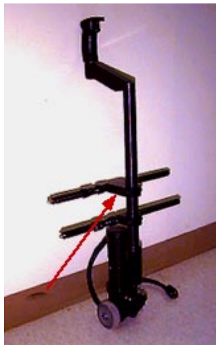
Figure 15. Suggestion for placement of the lower crossbar release mechanism (PICT, 133 k).
