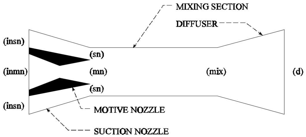
Figure 1.2 - Close-Up View Of Ejector
