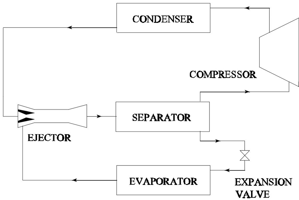
Figure 1.1 - Schematic of EERC
