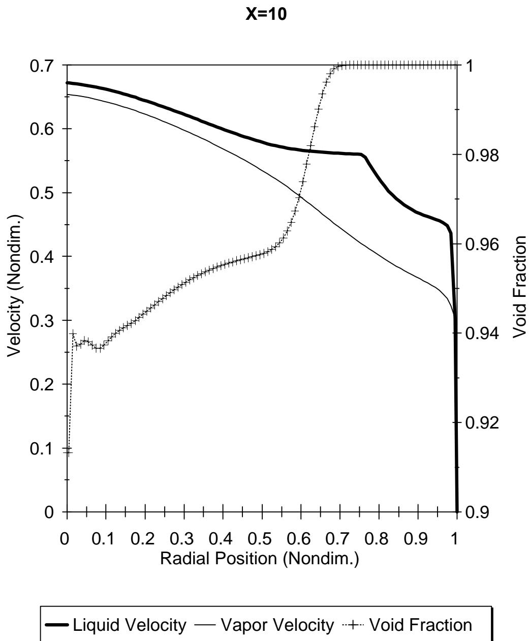
Figure 5.10 - Velocity Profile for Constant Droplet Diameter
