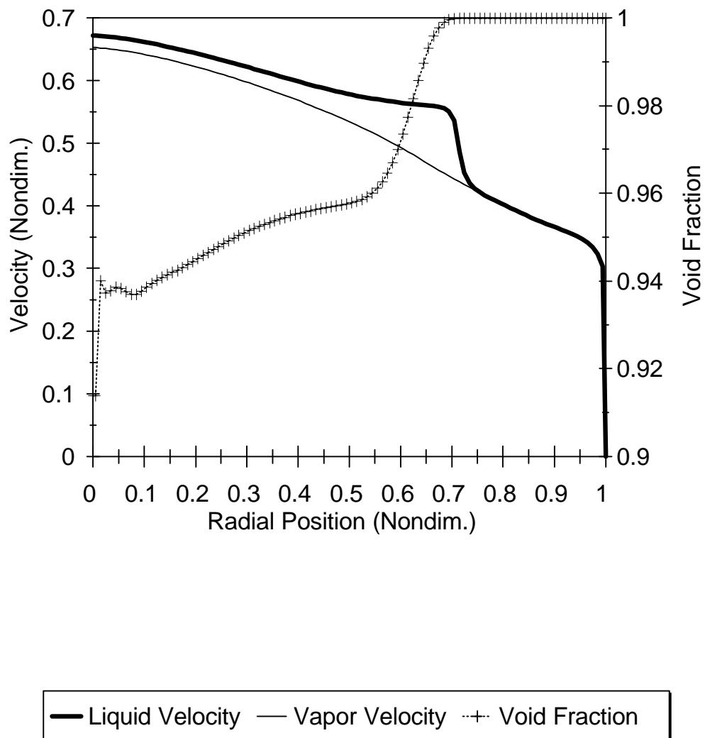
Figure 5.11 - Velocity Profile for Constant Droplet Diameter
