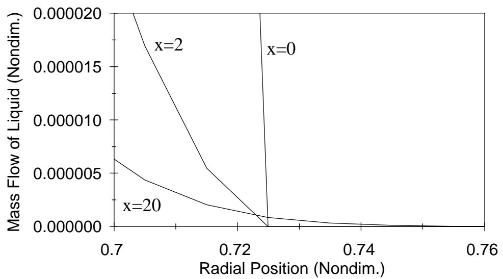
Figure 5.12 - Liquid Mass Distribution Across Domain with Closeup View
