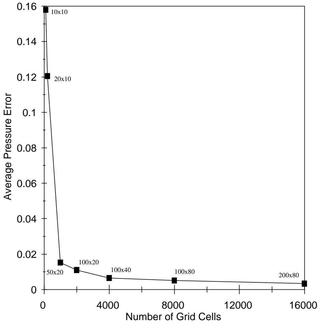
Figure 5.14 - Error Variation with Grid Refinement
