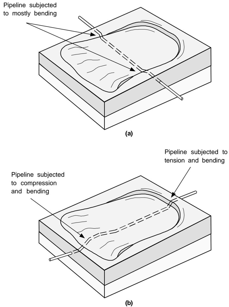
**Figure 3.2.** Pipeline damage in (a) perpendicular and (b) parallel crossings of a lateral spread (after O'Rourke and Lane 1989).
