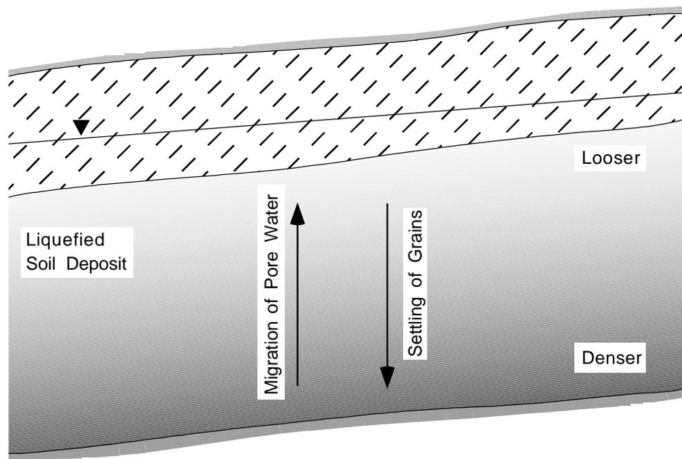
**Figure 3.4.** Settling of soil grains in a liquefied soil deposit leading to the upward migration of pore water (after *Liquefaction...* 1985).
