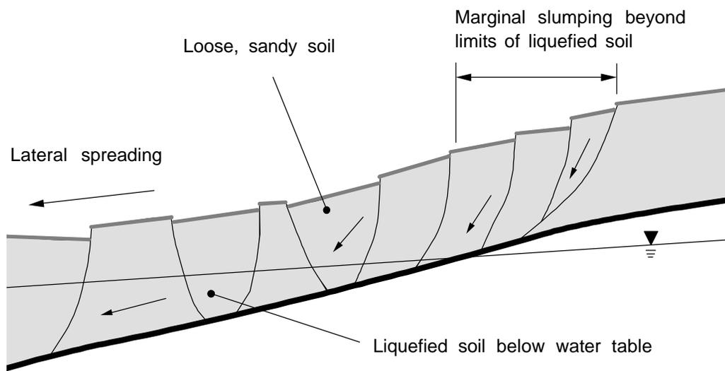
**Figure 3.6.** Marginal slumping around a lateral spread (after O'Rourke and Lane 1989).
