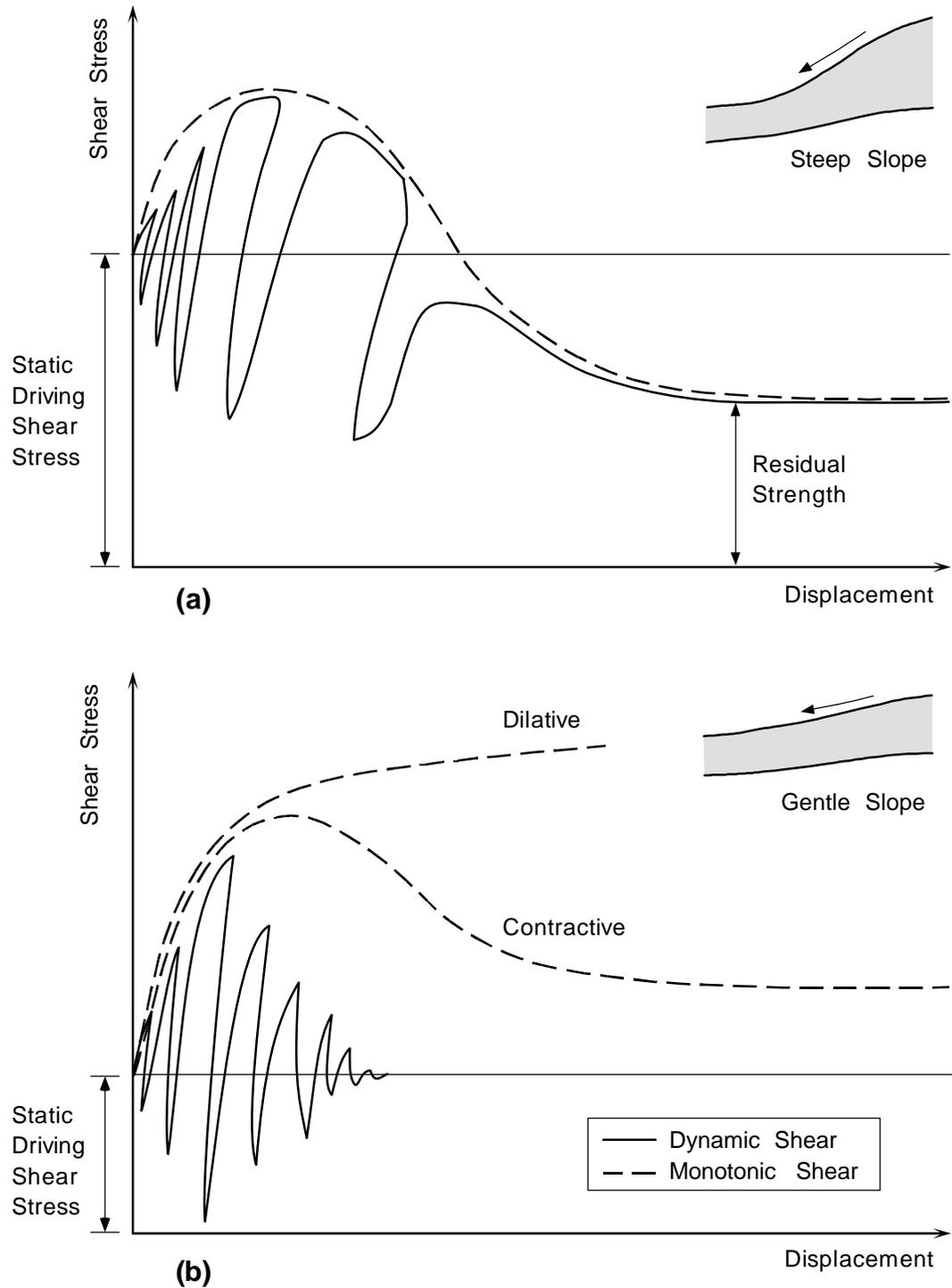
**Figure 3.3.** Earthquake-induced slope movements: (a) flow failure in a contractive soil, and (b) limited deformation in a dilative or contractive soil (after Ishihara 1994).
