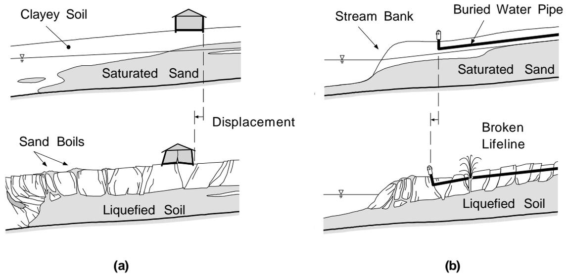
**Figure 3.1.** Soil liquefaction and lateral spreading of (a) gently sloping ground and (b) toward a free face.
