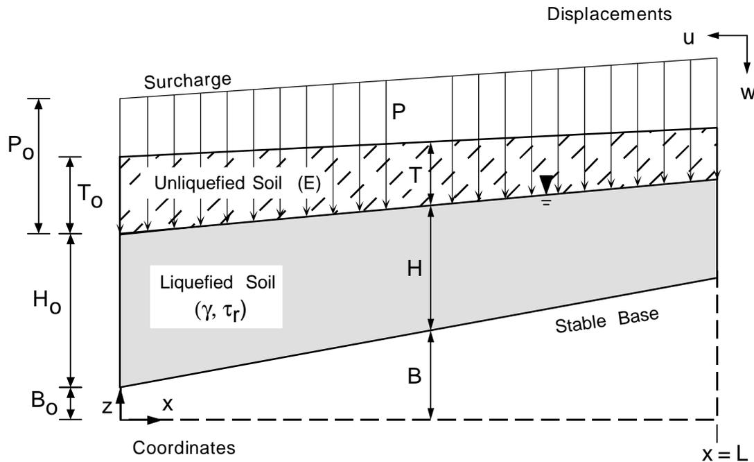
$B = B_0 + ax =$  thickness of stable base
