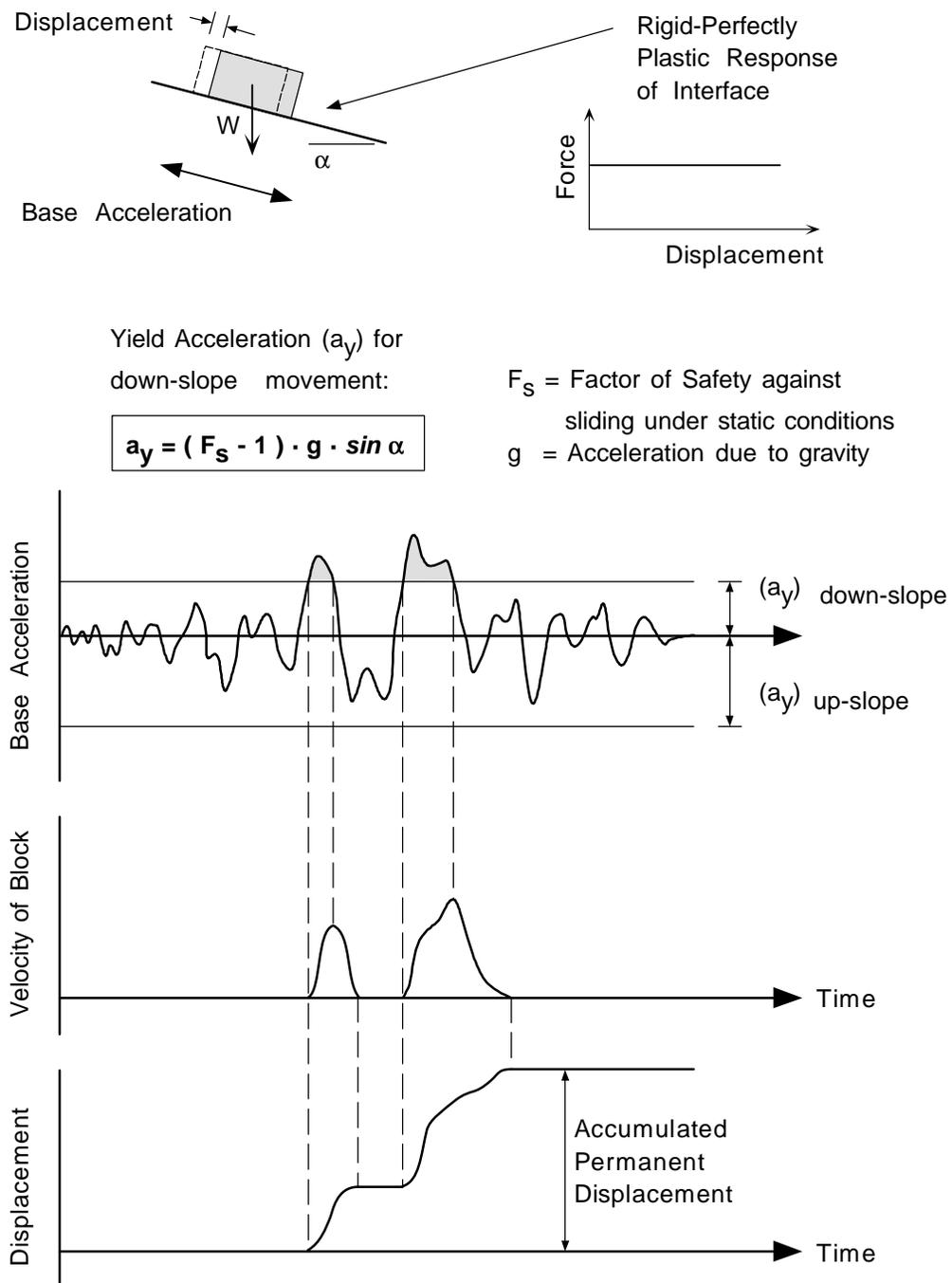
**Figure 4.1.** Calculation of displacements using Newmark's sliding block model (after Wilson and Keefer 1985).
