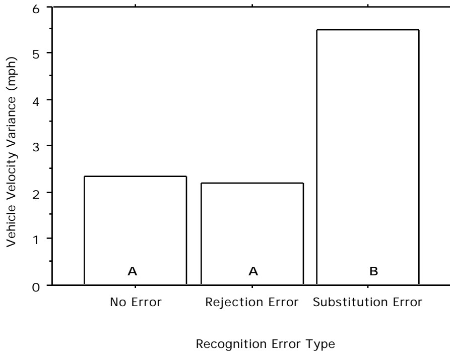
Figure 4. Mean vehicle velocity variance during task performance as a function of recognition error type. (Bold letters indicate significant differences in treatments. Treatments not sharing a common letter differ significantly from each other.)
