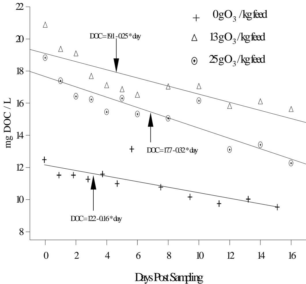
**Figure 2.8.** Batch tests indicated higher biological degradation rates of dissolved organic carbon (DOC) compounds in ozonated pilot scale recirculating aquaculture systems than in the unozonated system.
