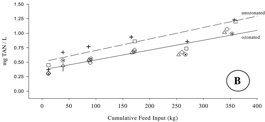
**Figure 2.4.** (A) Time profile of ambient environmental conditions in pilot scale recirculating aquaculture systems rearing market size hybrid striped bass receiving ozone treatment. Area denoted with arrows represents the period when feed consumption slowed and semi-continuous water exchanges occurred in the unozonated system. Plot (B) presents ambient TAN levels as a function of cumulative feed input between days 0 and 113 when water cumulative exchange rates were approximately equal.
