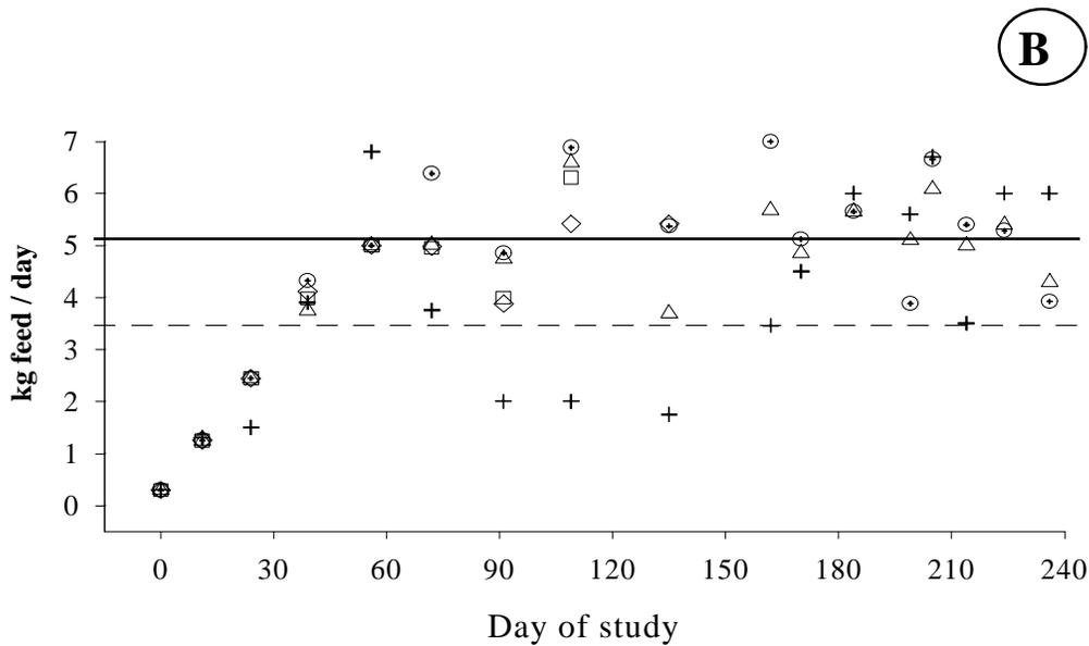
**Figure 2.3.** (A) Time profiles of cumulative feed inputs and fresh water replacements and (B) daily feed inputs (calculated at 7 day intervals) observed during the rearing of hybrid striped bass in pilot scale recirculating aquaculture systems receiving ozone injection. Solid and dotted horizontal lines mark the average daily feed delivered to the ozonated and unozonated systems, respectively.
