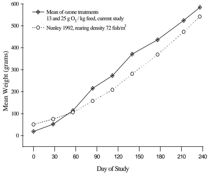
Figure 3.8. Mean weights of hybrid striped bass reared in an ozonated pilot-scale recirculating aquaculture systems at a stocking density of 150 fish/m<sup>3</sup> and hybrid striped bass reared in an unozonated recirculating system (Nunley 1992).
