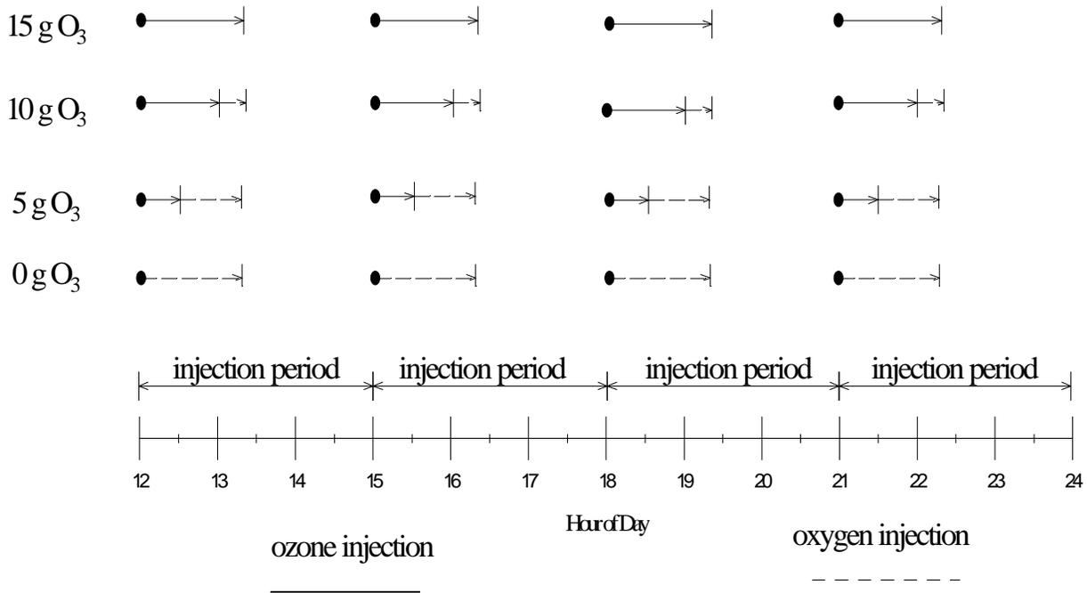
**Figure 2.A.1.** Presented is the ozone injection regime for the example and described in the in methods (ozone injection). The four injection periods denote the maximum time allowed, however in this problem the entire time was not required. Ozone would be injected at a rate of 10 g/hr at 4.8 lpm.
