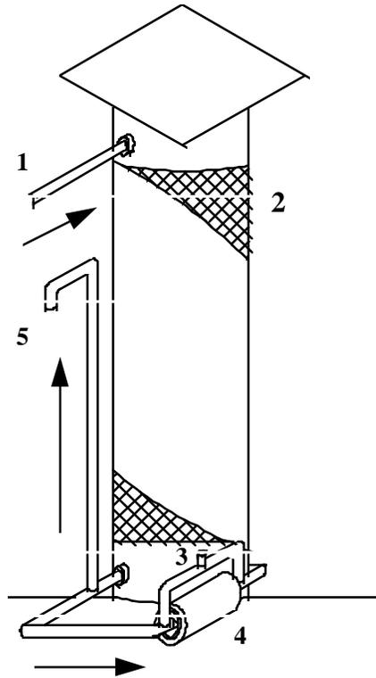
**Figure 2.2.** Ozone contactor used on a pilot scale recirculating aquaculture systems. Water entered through a port (1) positioned at the top of the contactor and flowed downward across packing material (2). Ozone / oxygen gas was aspirated into the contactor through a venturi injector (3) operated with a recirculation pump (4). Treatment was affected in countercurrent fashion, with water exiting (5) to biofilter.
