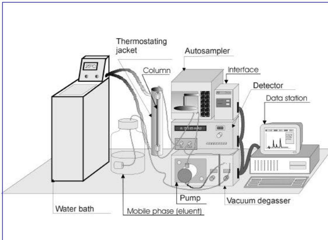
Figure 14. HPLC system with temperature control equipment.
