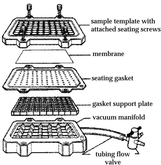
**Figure 2-4 Diagram of the assembly of the Bio-Dot apparatus. (Bio-Rad Instruction Manual)**
