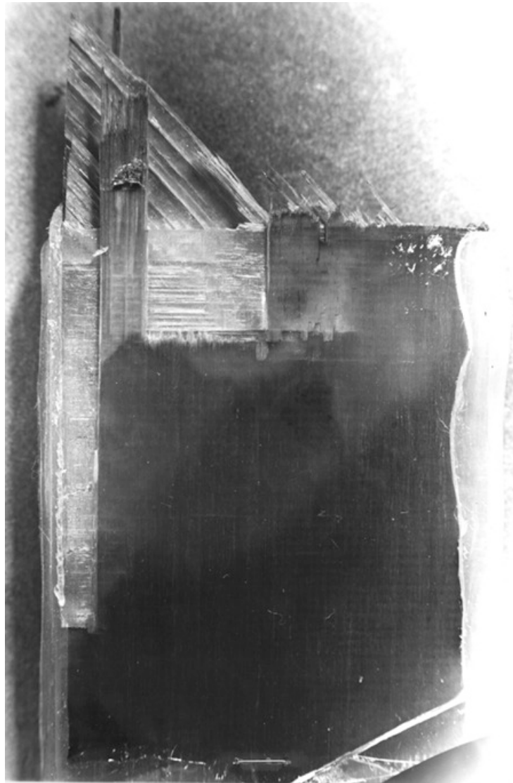
Figure 25. Representative fracture profile of stress-ruptured [0_2/90_2/+45_2/-45_2]_s E-Glass/913-epoxy having a lower stress (108 MPa), and shorter life (119 hours). The stress-corrosion cracks grow across about 20% of the laminate, while the 0^\circ plies cracked across much of the width before final separation.
