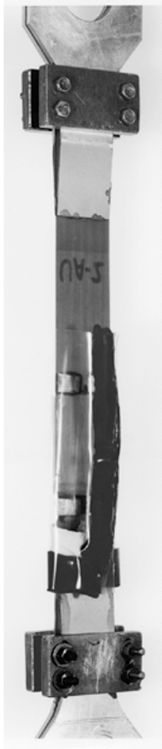
Figure 2(a). Unidirectional specimen showing clamps reinforcing the bonded end tabs. A clear plastic sheet is sealed with Tacky Tape brand of sealing strips to contain acid leaked from the acid cell upon failure of the specimen.
