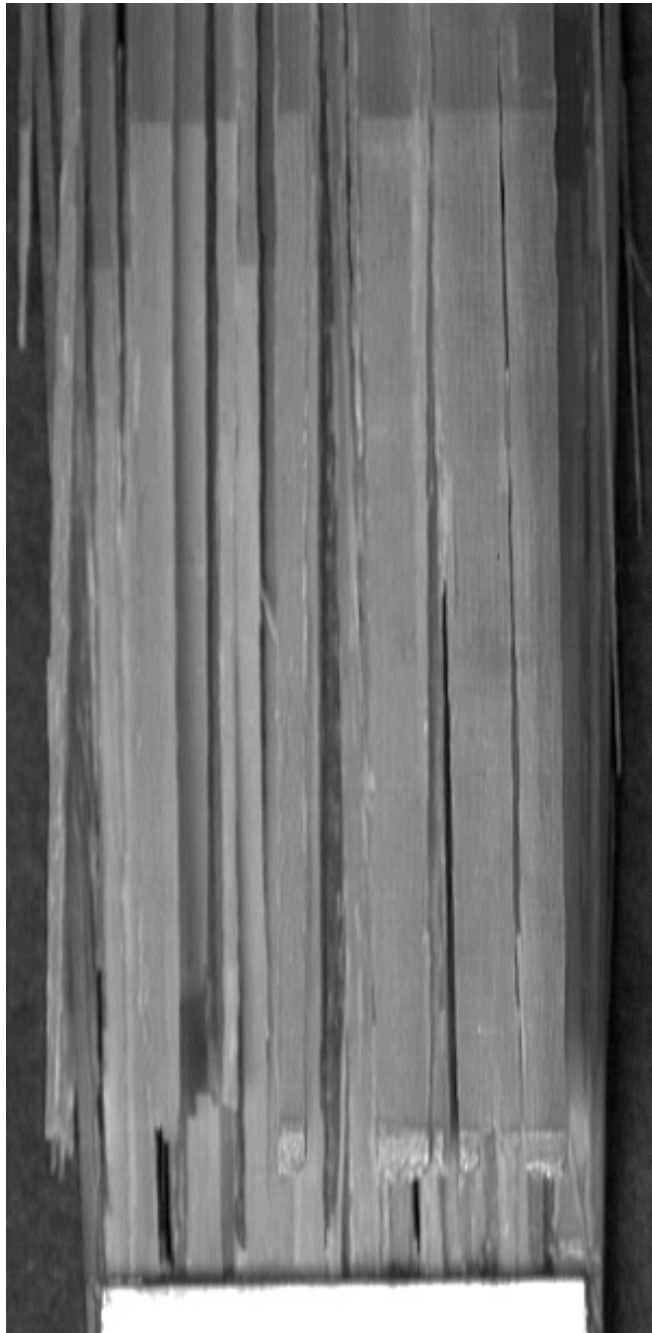
Figure 4(a). Fracture of [0]_8 quasi-static tensile specimen. Fracture initiated at the edge, at the grip edge, and proceeded by a repeated sequence of fiber fracture and splitting.
