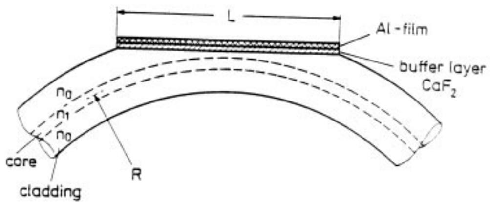
Figure 2.4 Side view of a fiber optic polarizer with buffer layer [76].
