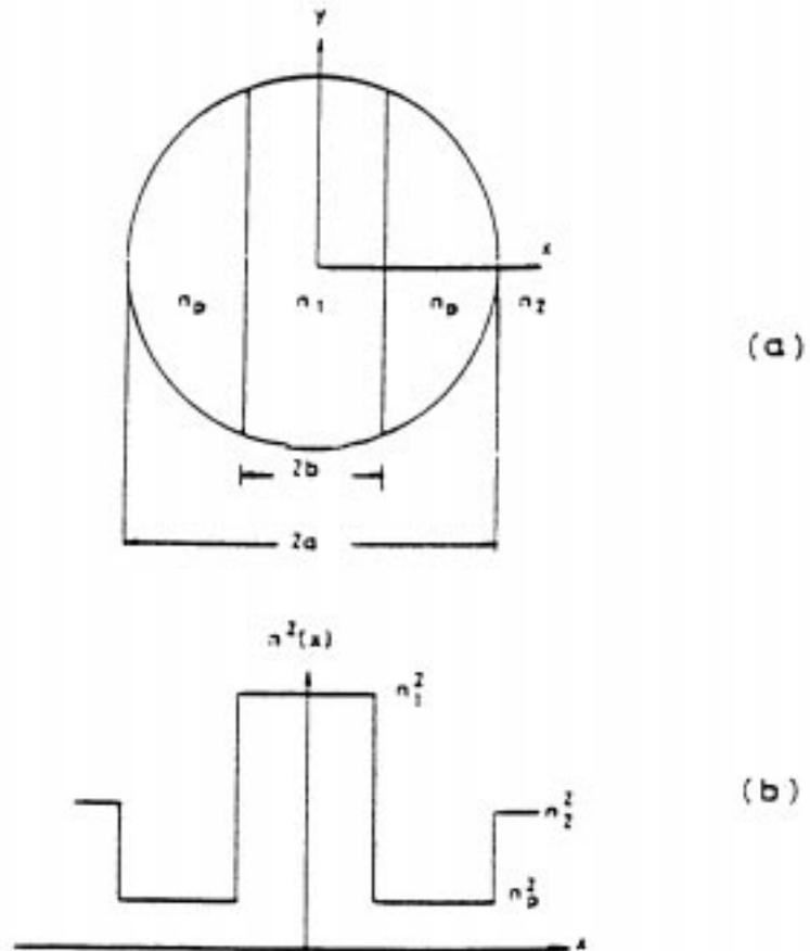
**Figure 2.2 Side-pit fiber (a) cross section, (b) refractive index distribution versus x-axis [4].**
