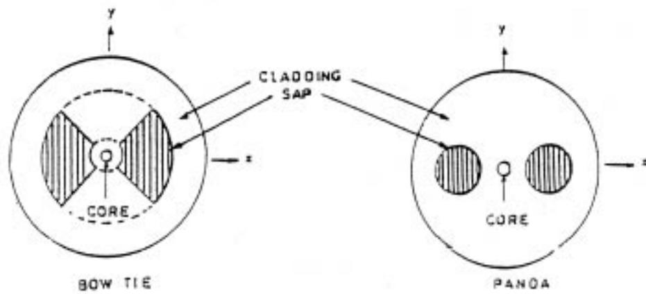
**Figure 2.3** Cross sections of Bow-tie and PANDA fibers [4].
