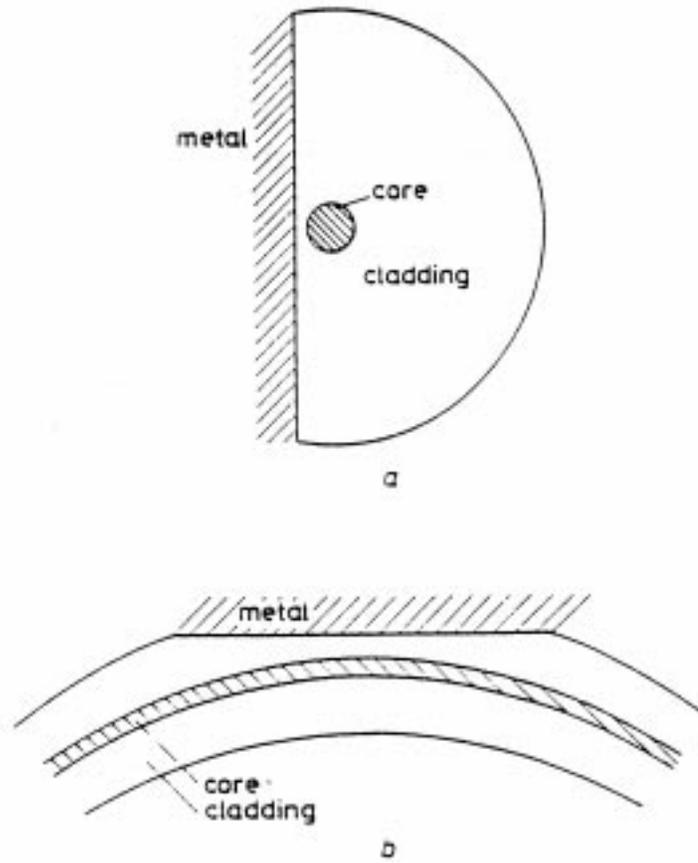
**Figure 2.5 A partial metal-clad fiber (a) cross section view of fiber optic polarizer, (b) side view of in-line fiber optic polarizer [17].**
