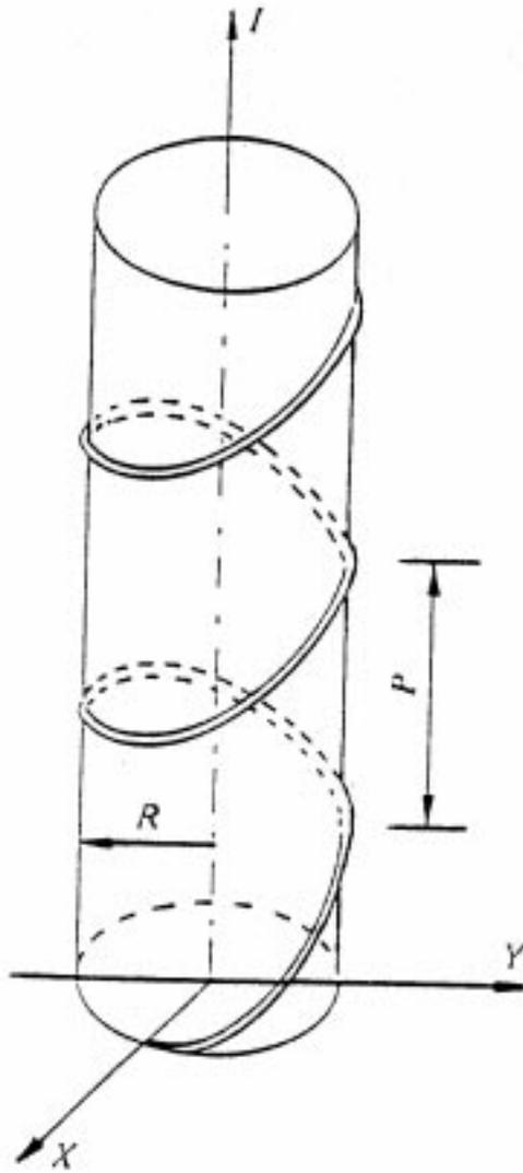
Figure 2.1 The structure of a helical or spiral fiber [23].
